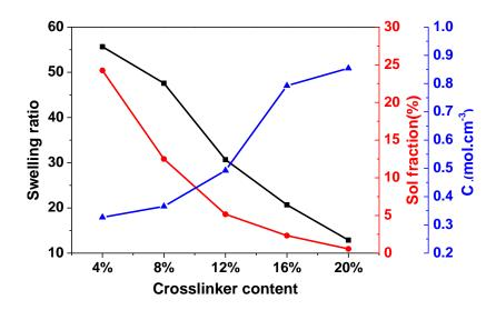
**Figure 3.** The cross-linking density, swelling ratio, and sol fraction of the C-FPAE series with different BDB contents.
