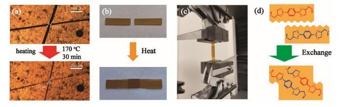
**Figure 8.** (a) Optical microscope images of self-healing performance for 20%C-FPEA. (b) Optical microscope images of welding performance. (c) Photograph of a sample during the lap-shear test. (d) Schematic representation of the transesterification reaction of boronic ester linkages.
