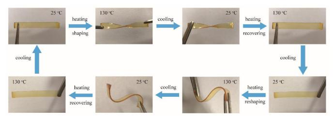
Figure 10. Optical microscope images of shape-memory performance of the 20% C-FPAE sample.
