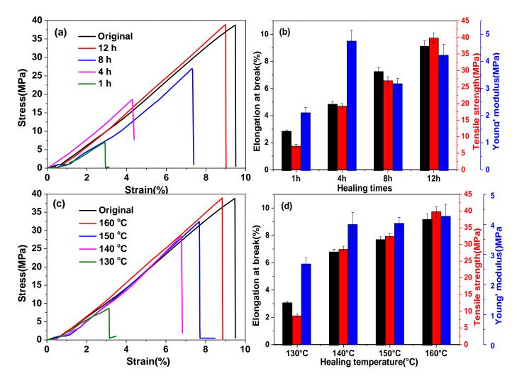
**Figure 9.** (a) Tensile curves of 20% C-FPEA welding at 160 °C for various times. (b) Mechanical properties of 20% C-FPEA welded at 160 °C for various times. (c) Tensile curves of 20% C-FPEA welding at 12 h for various temperatures. (d) Mechanical properties of 20% C-FPEA welded at 12 h for various temperatures.
