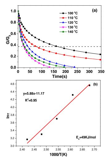
Figure 7. (a) Stress relaxation study of 20% C-FPAE. (b) Arrhenius plot with linear fit for 20% C-FPAE.
