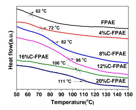
Figure 6. DSC curves of FPAE and C-FPAE series.
