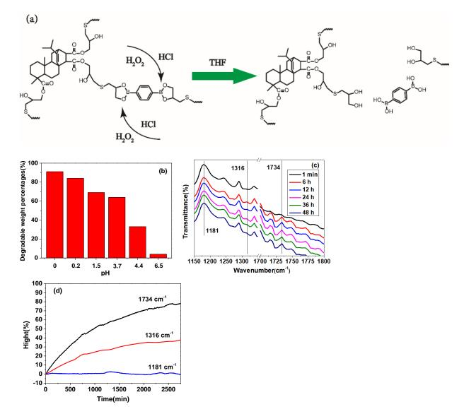
**Figure 12.** (a) Schematic representation of C-FPAE degradation. (b) The degradation weight percentage of 20% C-FPAE in mixed solutions with different pH. (c) Real-time FTIR spectra of 20% C-FPAE in mixed solution with pH = 0 for different times. (d) The height of the three characteristic peaks of FTIR (at 1734, 1316 and 1181 cm<sup>-1</sup>) during the degradation process.
