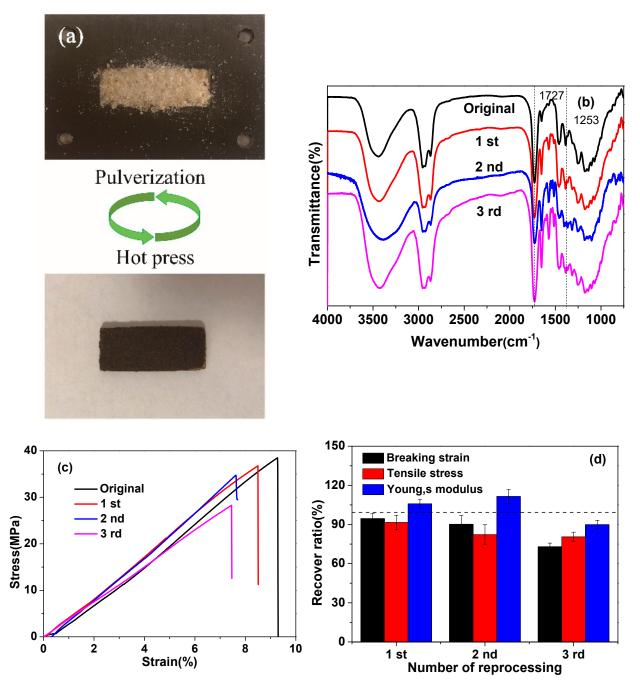
**Figure 11.** (a) Optical microscope images of thermal recycling performance of 20% C-FPAE by hot press. (b) FTIR spectra of 20% C-FPAE with different generations of reprocessing. (c) Tensile curves of samples with different generations of reprocessing. (d) Recovery ratios of samples with different generations of reprocessing.
