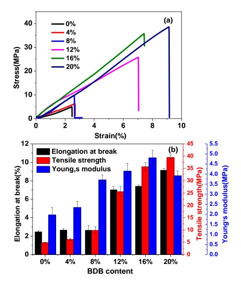
**Figure 4.** Mechanical properties of FPAE and C-FPAE series with different BDB contents: (**a**) stress–strain curve, (**b**) mechanical properties of the x% C-FPAE series with different cross-linker contents.
