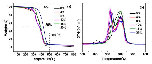
Figure 5. TGA (a) and DTG (b) curves of FPAE and C-FPAE series with different BDB contents.
