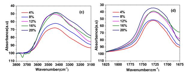
**Figure 2.** FTIR spectra of (**a**) BDB, FPAE, and 20% C-FPAE and (**b**) C-FPAE series with different BDB contents. (**c**) Hydroxyl and (**d**) carbonyl.
