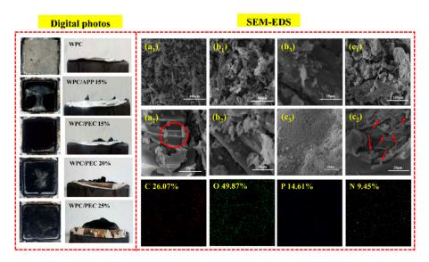
**Figure 5.** Digital photos of char residues from CCT, and their SEM images of WPC (**a**<sub>1</sub>,**a**<sub>2</sub>), WPC/APP 15% (**b**<sub>1</sub>,**b**<sub>2</sub>,**b**<sub>3</sub>), and WPC/PEC 15% (**c**<sub>1</sub>,**c**<sub>2</sub>,**c**<sub>3</sub>) and its EDX pattern of char residues.
