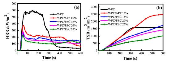
Figure 3. CCT results of WPC with PEC: (a) HRR and (b) TSR.
