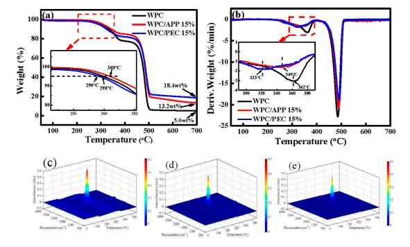
**Figure 4.** Thermal results of WPC with APP and PEC: TG (**a**) and DTG (**b**) curves, and the 3D-FTIR spectra of the volatile pyrolysis products from room temperature to 700 °C during the whole pyrolysis: WPC (**c**), WPC/APP 15% (**d**), WPC/PEC 15% (**e**).
