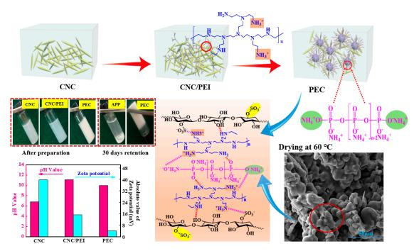
**Figure 1.** Fabrication schematic diagram of polyelectrolyte complex (PEC) based on cellulose nanocrystals (CNC), polyethyleneimine (PEI), and ammonium polyphosphate (APP), and its storage stability, pH values, and zeta potential values.
