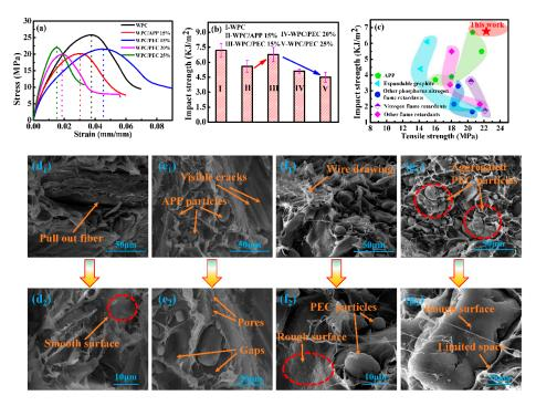
**Figure 7.** Mechanical properties and fractural morphology of WPC with APP and PEC: (**a**) Strain–stress curves, (**b**) impact strength, and (**c**) comparison with other reported flame retardants [2,26–32]. SEM images of WPC (**d**<sub>1</sub>,**d**<sub>2</sub>), WPC/APP 15% (**e**<sub>1</sub>,**e**<sub>2</sub>), WPC/PEC 15% (**f**<sub>1</sub>,**f**<sub>2</sub>), and WPC/PEC 25% (**g**<sub>1</sub>,**g**<sub>2</sub>).
