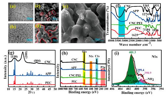
**Figure 2.** Morphological and physicochemical characterization of PEC. TEM of CNC (**a**) and APP (**b**), SEM of APP (**c**), PEC (2000×, **d**), and PEC (4000×, **e**), FTIR (**f**), XRD (**g**), XPS (**h**) spectra of PEC, and its N1s high-resolution spectra of PEC (**i**).
