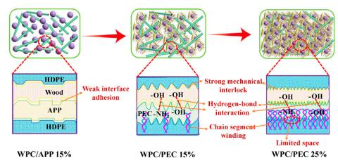
Figure 8. PEC distribution within WPC and possible interfacial bonding mechanisms.
