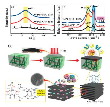
**Figure 6.** Chemical structure of char residues: XRD (**a**) and Raman spectra (**b**), and possible flame retardancy mechanism of WPC with PEC (**c**).
