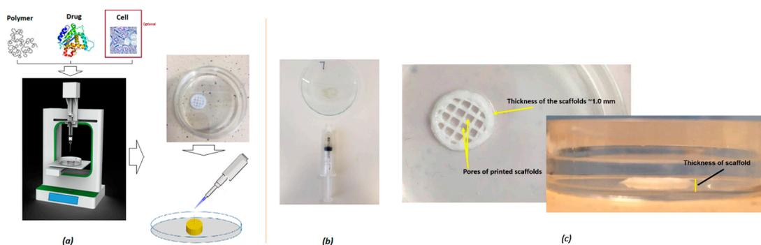
**Figure 1.** Schematic diagram of (a) the optimized 3D bioprinting process, (b) the extrudable bioink, and (c) the printed scaffold with 3D texture.
