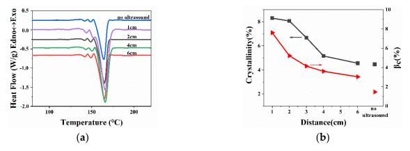
**Figure 8.** (a) The melting behaviors of WBG-PP at different ultrasound distances. (b) Effect of the ultrasound distance on the values of relative content of the  $\beta$ -crystal form ( $\beta_c$ ) and crystallinity ( $\theta$ ).
