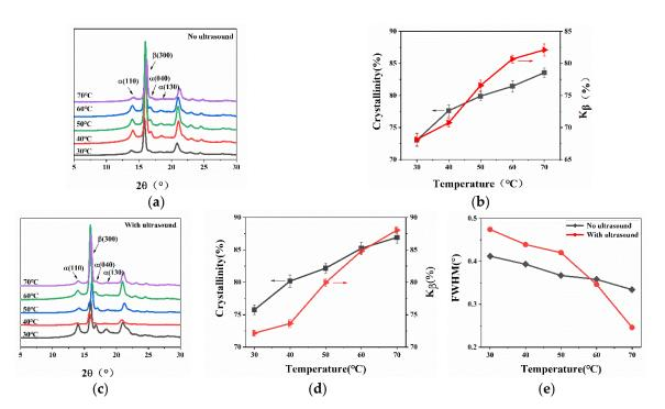
**Figure 10.** (**a**) XRD atlas of WBG-PP without ultrasound. (**b**) The  $w_{c,x}$  and  $K_{\beta}$  values of WBG-PP without ultrasound. (**c**) XRD atlas of WBG-PP with ultrasound. (**d**) The  $w_{c,x}$  and  $K_{\beta}$  values of WBG-PP with ultrasound. (**e**) Contrast of the FWHM of the diffraction peaks on the  $\beta$ -crystal plane with and without ultrasound.
