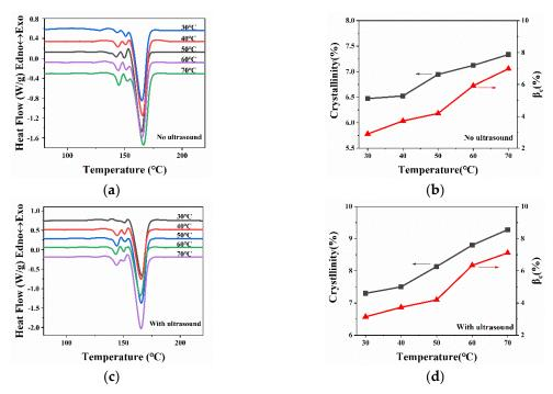
**Figure 11.** (a) The melting behaviors of WBG-PP under different cooling temperatures. (b) Effect of the cooling temperature on the values of  $\beta_c$  and  $\theta$ . (c) The melting behaviors of WBG-PP under different cooling temperatures with ultrasound. (d) Effect of the cooling temperature with ultrasound on the values of  $\beta_c$  and  $\theta$ .
