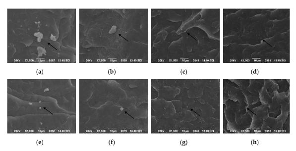
**Figure 5.** Dispersion of the nucleating agent under different cooling temperatures without ultrasound: (a) 30 °C, (b) 40 °C, (c) 50 °C, (d) 60 °C; and with ultrasound: (e) 30 °C, (f) 40 °C, (g) 50 °C, (h) 60 °C.
