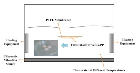
**Figure 2.** Device diagram of  $\beta$ -nucleating agent polypropylene (WBG-PP) thin film prepared by ultrasound.
