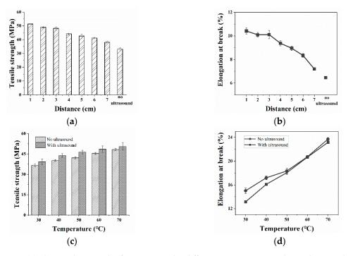
**Figure 12.** (a) The tensile strength of WBG-PP under different temperatures without ultrasound and with ultrasound. (b) The elongation at the break of WBG-PP under different temperatures without ultrasound and with ultrasound. (c) The tensile strength of WBG-PP at different ultrasound distances. (d) The elongation at the break of WBG-PP at different ultrasound distances.
