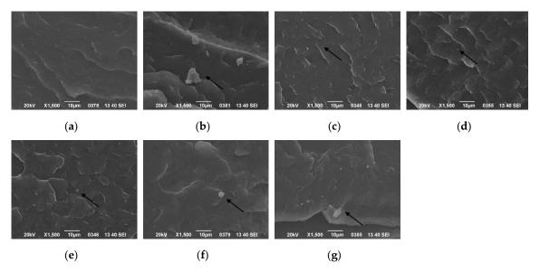
**Figure 4.** Effect of different ultrasound distances on dispersion of the nucleating agent in the PP matrix: (a) pure PP; (b) without ultrasound; (c) 1 cm; (d) 2 cm; (e) 3 cm; (f) 5 cm; (g) 7 cm.
