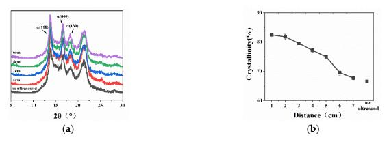
**Figure 6.** (a) Wide-angle X-ray diffraction pattern of pure PP prepared at different ultrasound distances. (b) Changes in the crystallinity ( $w_{c,x}$ ).
