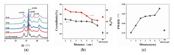
**Figure 7.** (a) Wide-angle X-ray diffraction pattern of WBG-PP prepared at different ultrasound distances. (b) Changes in the crystallinity ( $w_{c,x}$ ) and the relative content of  $\beta$ -crystals ( $K_{\beta}$ ). (c) Changes in the full width at half maximum (FWHM) of the  $\beta$  (300) crystal plane.
