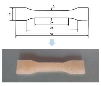
Figure 3. Shape and dimensions of a standard tensile spline.
