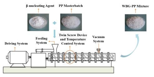
**Figure 1.** Process flow chart of preparing  $\beta$ -nucleating agent polypropylene (WBG-PP) using a twinscrew extruder.
