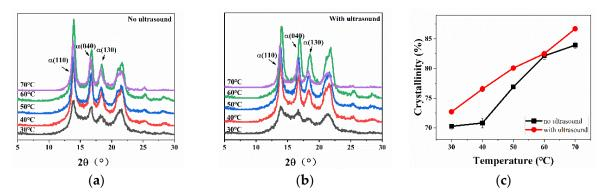
**Figure 9.** (a) X-ray diffraction (XRD) atlas of pure PP without ultrasound. (b) XRD atlas of pure PP with ultrasound. (c) The  $w_{c,x}$  values of pure PP without ultrasound and with ultrasound.
