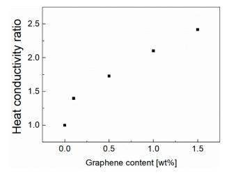
**Figure 9.** The variation of the heat conductivity ratio of the membranes as a function of the graphene content.
