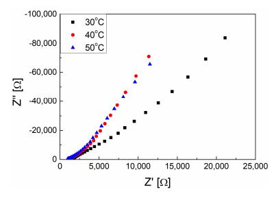
Figure 4. The Nyquist plots of 0.1 mol/L KCl solution at 30, 40, and 50 °C, respectively.
