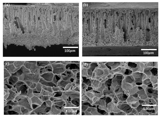
**Figure 2.** SEM cross-section of the PVDF/1% graphene membrane as prepared samples (**a**,**c**) as well as the samples after being immersed in hot water (**b**,**d**).
