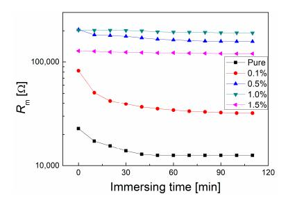
**Figure 7.** The plots of membrane resistance vs. immersing time for different PVDF membranes immersing 0.1 mol/L KCl solution at 30 °C.
