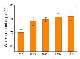
Figure 3. Water contact angle of the membranes.
