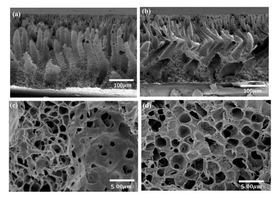
**Figure 1.** SEM cross-section of the PVDF membrane as prepared samples (**a**,**c**) as well as after the samples were immersed in hot water (**b**,**d**).
