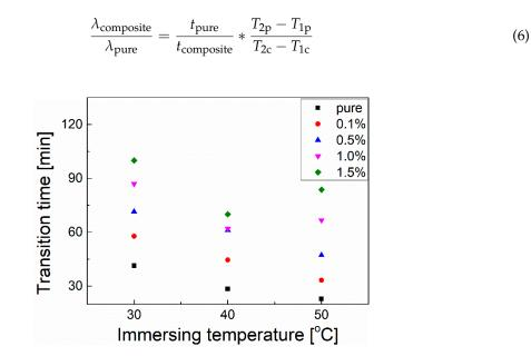
**Figure 8.** The transition time vs. the immersing temperature for the membranes immersed in the solution.
