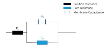
Figure 6. The equivalent circuit model for the present system.
