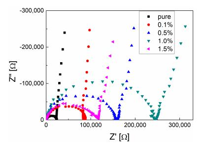
**Figure 5.** The Nyquist plot of the PVDF membrane with different graphene contents immersing in 0.1 mol/L KCl solution at room temperature.
