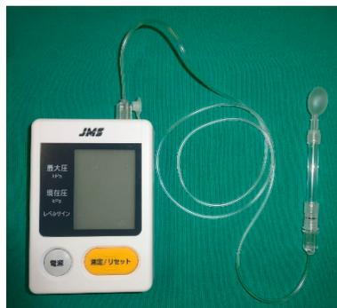
Figure 6. Digital tongue pressure meter.
