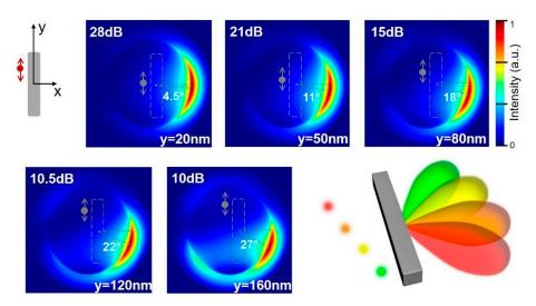
**Figure 3.** The influence of lateral displacement on radiation direction. Angular emission patterns with different dipole y-positions at 660 nm. The F/B values and the deflection angle of the emission lobe are also shown. The cartoon illustrates a brief description of the possible implementation of an integrated nanodevice for angle-resolved color routing.
