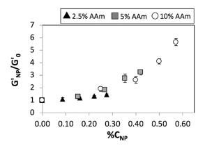
**Figure 4.** Relative elastic moduli of 2.5% pAAm (white circles), 5% pAAm (grey squares), and 10% pAAm (black triangles) hydrogels prepared using  $%C_{Bis} = 4.76$  as a function of relative nanoparticle concentration ( $%C_{NP}$ ). Data shown are the mean of triplicate measurements  $\pm$  standard deviation and have been repeated at least three times with similar results.
