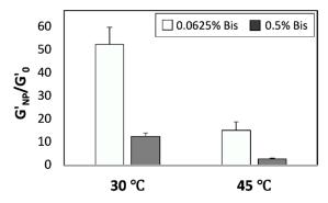
**Figure 5.** Relative elastic moduli of 5% pNIPAAm hydrogels prepared using 0.0625% Bis (white bars) or 0.5% Bis (grey bars), and 5% SiNPs at different temperatures. Data shown are the mean of triplicate measurements plus standard deviation and have been repeated at least three times with similar results.
