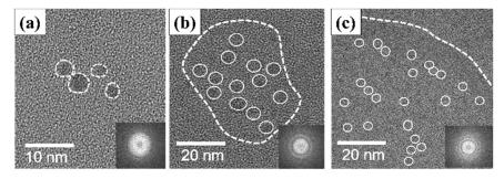
**Figure 2.** HR-TEM micrographs of (**a**) GQD-P, (**b**) GQD-6k, and (**c**) GQD-100k samples, where the inset shows their corresponding SAD patterns.
