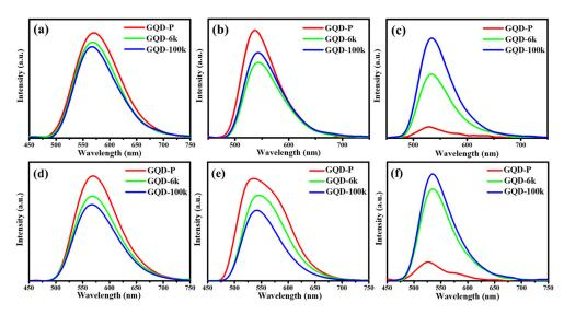
**Figure 7.** PL emission spectra of pristine GQD and PEG-coated GQD cluster suspensions in (**a**) water, (**b**) ethanol, and (**c**) PGMEA under an excitation of 360 nm. PL emission spectra of pristine GQD and PEG-coated GQD cluster suspensions in (**d**) water, (**e**) ethanol, and (**f**) PGMEA under an excitation of 450 nm.
