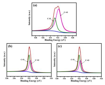
**Figure 5.** XPS O1s spectra of (**a**) GQD-P, (**b**) GQD-6k, and (**c**) GQD-100k samples, decomposed by a multiple Gaussian function.
