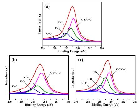
**Figure 3.** XPS C1s spectra of (**a**) GQD-P, (**b**) GQD-6k, and (**c**) GQD-100k samples, decomposed by a multiple Gaussian function.
