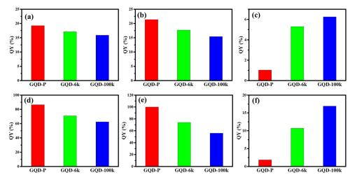
**Figure 8.** The QY values of pristine GQD and PEG-coated GQD cluster suspensions in (**a**) water, (**b**) ethanol, and (**c**) PGMEA under an excitation of 360 nm. The QY values of pristine GQD and PEG-coated GQD cluster suspensions in (**d**) water, (**e**) ethanol, and (**f**) PGMEA under an excitation of 450 nm.
