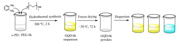
Figure 1. Schematic of PEG-coated GQD clusters (GQD-6k) through one-pot hydrothermal route.
