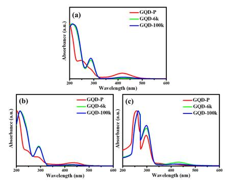
**Figure 6.** UV-vis absorbance spectra of pristine GQD and PEG-coated GQD cluster suspensions in (a) water, (b) ethanol, and (c) PGMEA.
