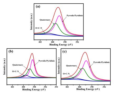
**Figure 4.** XPS N1s spectra of (**a**) GQD-P, (**b**) GQD-6k, and (**c**) GQD-100k samples, decomposed by a multiple Gaussian function.
