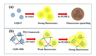
**Figure 9.** Schematic diagram for the PL emission from (**a**) GQD-P and (**b**) GQD-100k suspensions in different solvents under blue-light illumination.
