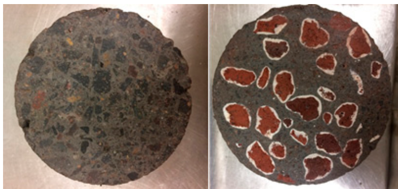
Figure 15. Cross section of control and TESA samples.
