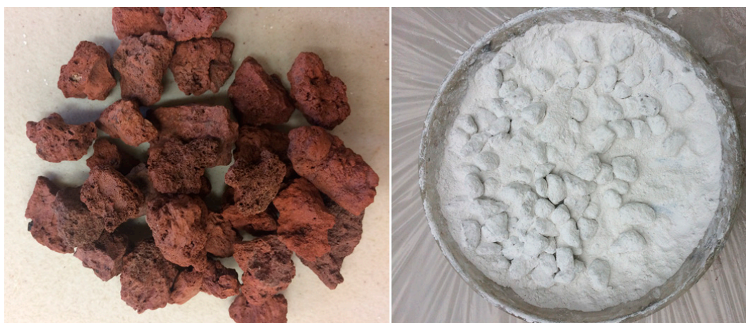
Figure 14. Scoria before and after coating.
