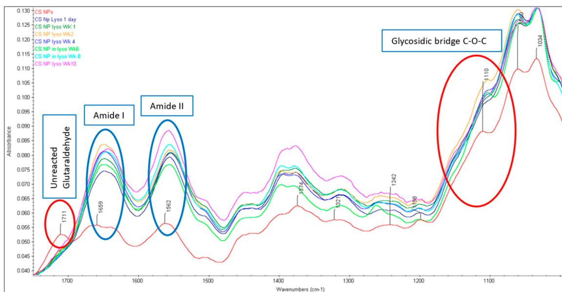
**Figure 3.** FTIR spectra of CS NPs before and after lysozyme treatment (characteristic peaks for amide I, II and glycosidic bonds are highlighted).
