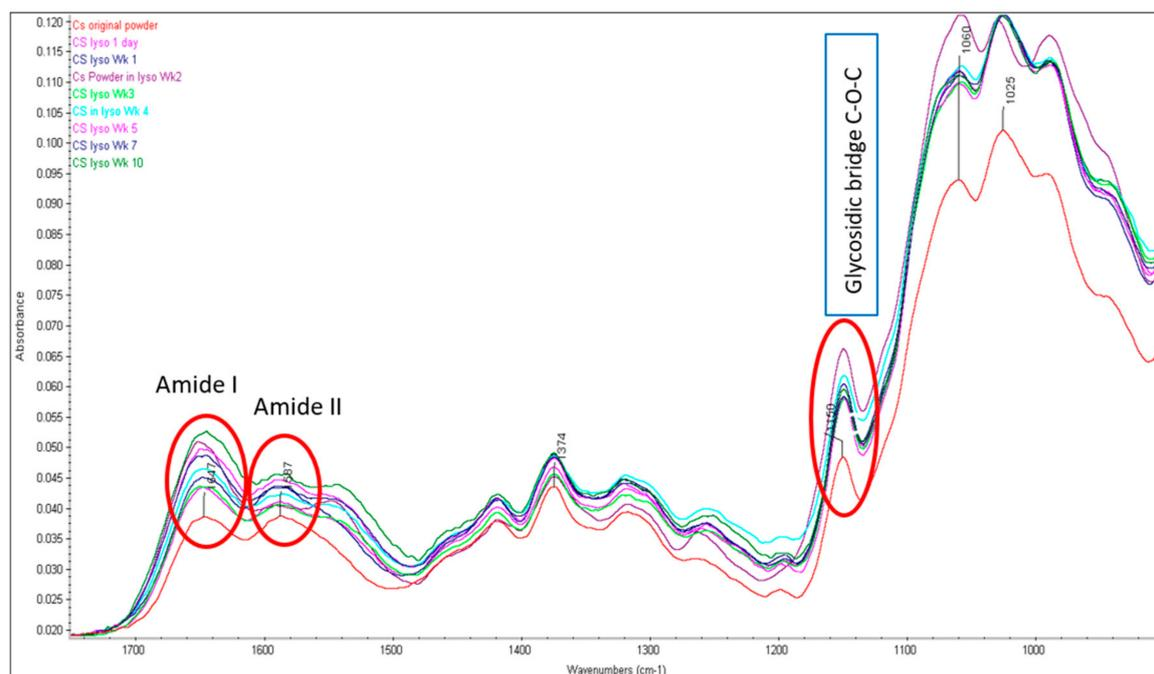
**Figure 2.** FTIR spectra of CS powders before and after lysozyme treatment (characteristic peaks for amide I, II and glycosidic bonds are highlighted).
