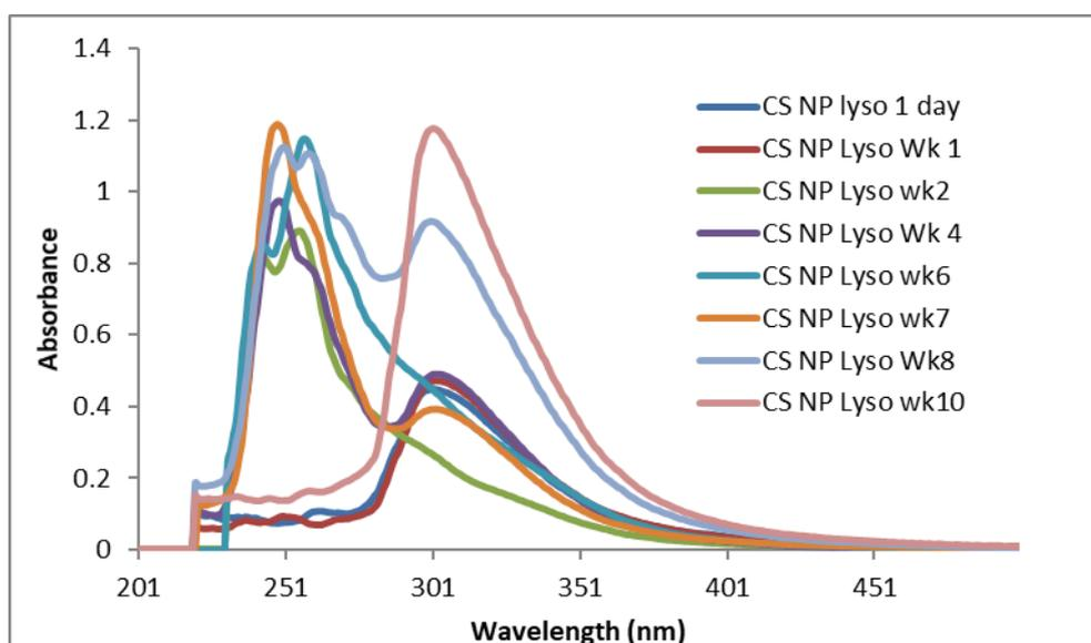
**Figure 10.** UV- Vis spectra of the supernatant of CS NPs incubated in 0.2% lysozyme solution at 37 °C.
