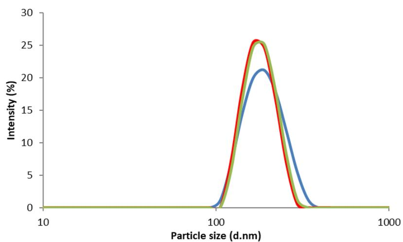
**Figure 6.** Particle size and size distributions of CS NPs.
