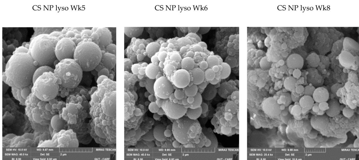
**Figure 5.** SEM images of CS NPs before and after incubating in 0.2 mg/mL lysozyme solution at different time intervals.
