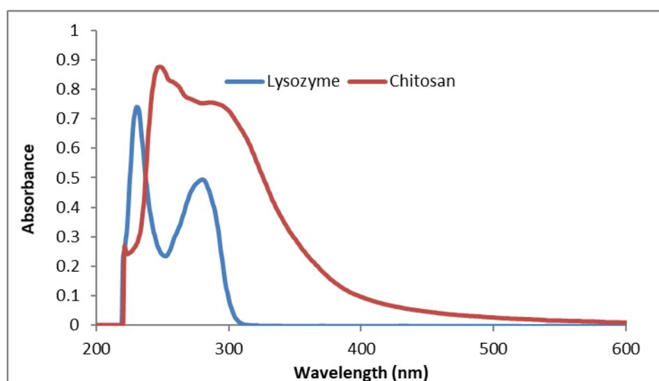
**Figure 8.** UV-VIS spectra of CS solution (1.0% *w/v*) in acetic acid (1% *v/v*) and lysozyme solution (0.2 mg/mL) in PBS (pH 7.4).
