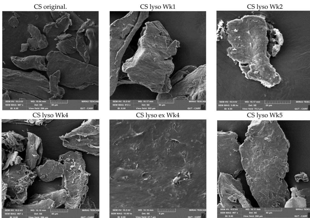
**Figure 4.** SEM images of CS before and after incubating in 0.2 mg/mL lysozyme solution at different time intervals.
