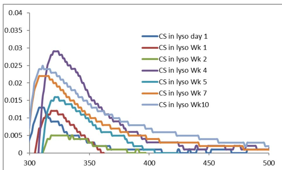
**Figure 9.** UV-VIS spectra of CS original powder incubated in 0.2% lysozyme solution at 37 °C.
