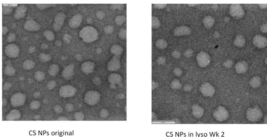
**Figure 7.** TEM images of CS NPs before and after incubating in 0.2 mg/mL lysozyme solution at 37 °C (TEM images for samples incubated up to 10 weeks could not be performed).
