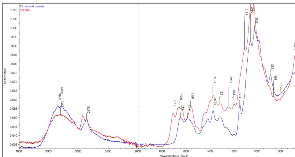
**Figure 1.** FTIR spectra of CS original powder and CS NP before incubating in 0.2 mg/mL lysozyme solution.
