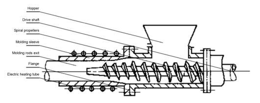
Figure 6. Schematic diagram of the briquetting equipment.
