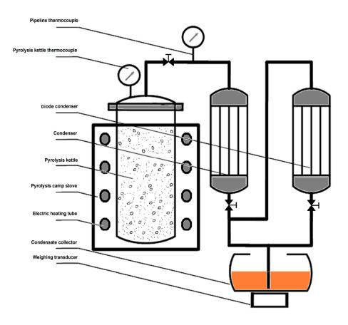
Figure 7. Schematic diagram of the pyrolysis equipment.
