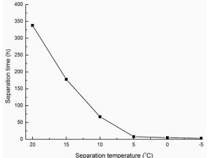
Lower cooling temperatures gave better separation of the two phases than higher temperatures, and this reduced the separation time. Separation of the condensate at 20 °C required nearly 350 h for complete separation. The separation rate was higher below 5 °C, and the condensate was completely
