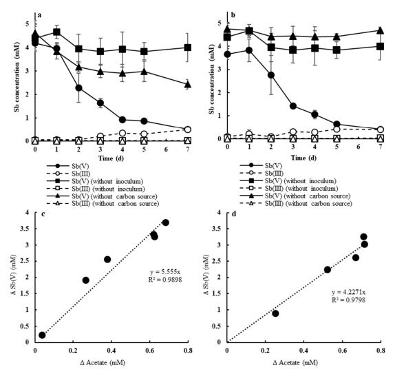
**Figure 1.** Time course of soluble Sb(V) and Sb(III) (**a**,**b**) and the relationship between acetate consumption ( $\Delta$ Acetate) and Sb(V) decline ( $\Delta$ Sb(V)) (**c**,**d**) during anaerobic Sb(V) reduction by strains AR-2 (**a**,**c**, respectively) and AR-3 (**b**,**d**, respectively). Error bars represent the standard deviation (*n* = 3).
