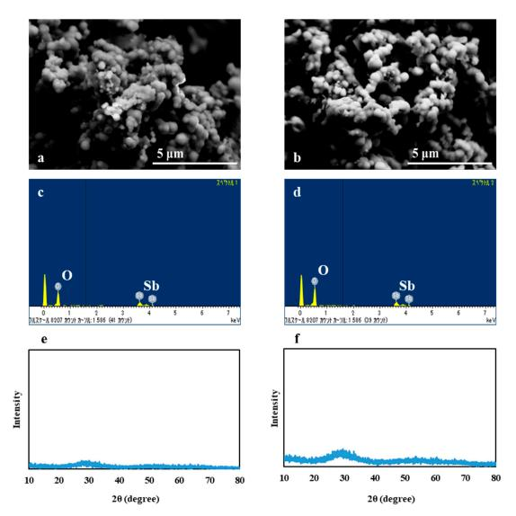
**Figure 3.** Scanning electron micrographs (**a**,**b**), energy-dispersive X-ray spectroscopy spectra (**c**,**d**), and X-ray diffraction patterns (**e**,**f**) of precipitates formed during anaerobic Sb(V) reduction for 7 d by strains AR-2 (**a**,**c**,**e**, respectively) and AR-3 (**b**,**d**,**f**, respectively).
