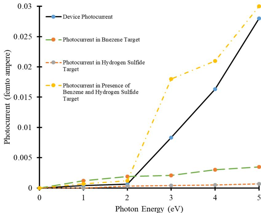
**Figure 6.** Photon energy vs. photocurrent curves of carbon nanotube-based device in presence of benzene and hydrogen-sulfide target molecules.
