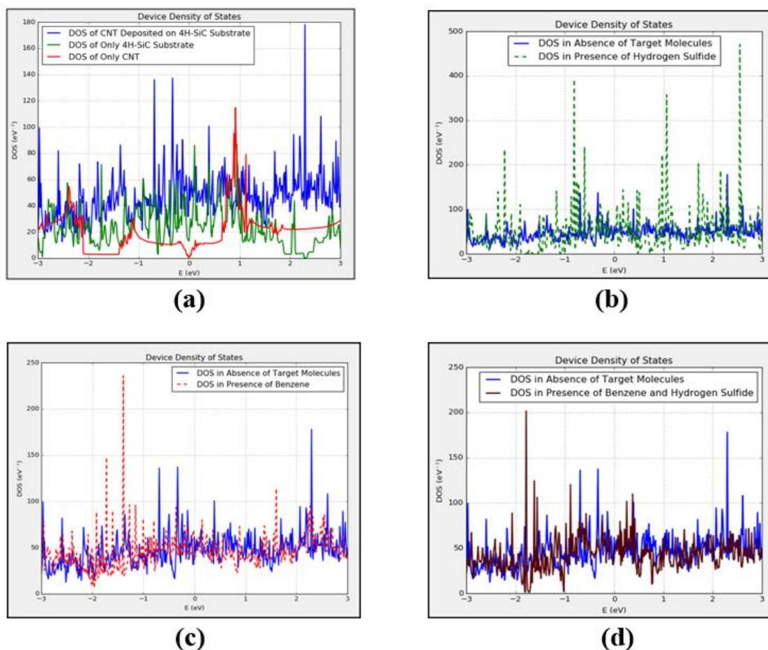
**Figure 3.** Density of states (DOS) of (a) only carbon nanotube-based device; (b) device in presence of only hydrogen-sulfide molecules; (c) device in presence of only benzene molecules; (d) device in presence of both hydrogen-sulfide and benzene molecules.
