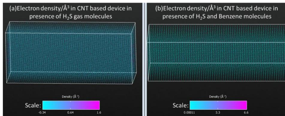
**Figure 5.** Electron density/ $\text{\AA}^3$  of simulated device in presence of (a) only  $\text{H}_2\text{S}$  gas molecules; (b) both  $\text{H}_2\text{S}$  and benzene molecules.
