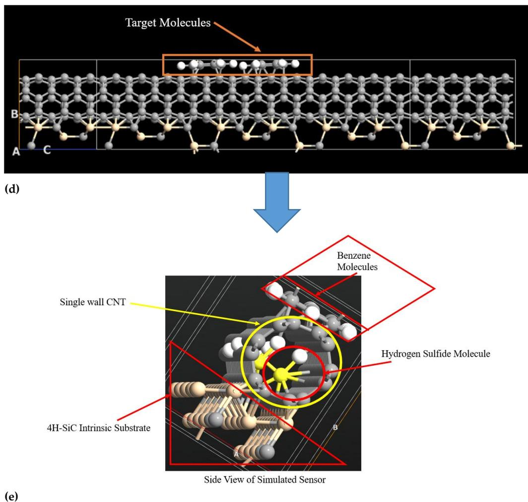
**Figure 1.** Simulation of single-wall carbon nanotube-based hydrogen-sulfide and benzene detector in Quantumwise Atomistix Toolkit Software.
