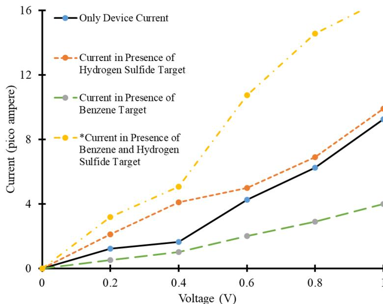
**Figure 4.** Current-voltage ( $I$ - $V$ ) curves of carbon nanotube based simulated device in the proximity of benzene and hydrogen-sulfide as target molecules (\*multiply current axis with  $10^6$  to get the exact value of current in pico ampere for benzene and hydrogen-sulfide target curve).
