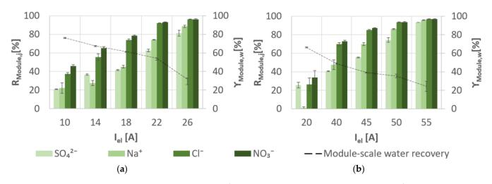
**Figure 7.** Specific module-scale salt rejection ( $R_{Module,j}$ ) and module-scale water recovery ( $\gamma_{Module,w}$ ) for experimental desalination: (**a**) slightly SGW and (**b**) moderately SGW using MCDI.
