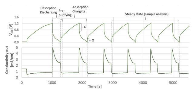
**Figure 6.** Cell voltage ( $V_{cell}$ ) and conductivity of the outflow of the MCDI module during desalination of slightly SGW at 14 A ( $\Omega$ : ohmic resistance).
