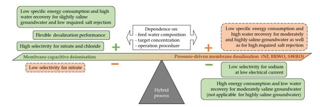
**Figure 8.** Benefits and drawbacks of pressure-driven membrane desalination (red and dashed frame) and membrane capacitive deionisation (green and solid frame) detected in this study.
