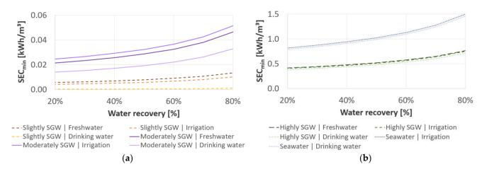
**Figure 2.** Minimum volume-related specific energy consumption ( $SEC_{min,V}$ ) as a function of water recovery: (**a**) for slightly SGW and moderately SGW; (**b**) for highly SGW and seawater regarding the target concentrations for fresh groundwater, water for irrigation and drinking water.
