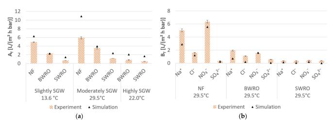
**Figure 3.** Average permeability: (a) water permeability ( $A_T$ ), (b) salt permeability ( $B_T$ ) for desalination of moderately SGW at 29.5 °C. The bars show the 95% confidence interval for the experimental results. NF: nanofiltration; BWRO: brackish water reverse osmosis; SWRO: seawater reverse osmosis.
