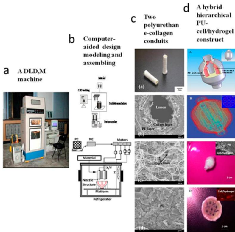
**Figure 6.** A double-nozzle low-temperature (DLDM) technology developed at Tsinghua University, prof. Wang' group: (a) the DLDM printer; (b) schematic description of the working processes of the two nozzles; (c) a tubular polyurethane-collagen conduit made by the DLDM system; and (d) an elliptical hybrid hierarchical polyurethane and cell/hydrogel construct made by the DLDM system [12].
