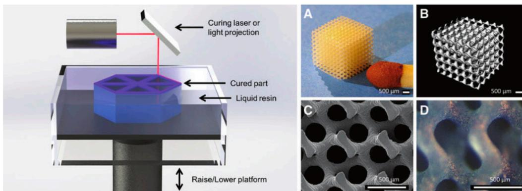
**Figure 4.** Schematic of stereolithographic (SLA) printing technique; and (A–D) exemplary tissue engineering scaffold composed of poly(D-L lactic acid) (PDLA) that showcases the resolution and detail of SLA [47]: (A) photograph; (B) micro computed tomography (mCT); and (C,D) scanning electron microscope (SEM). Scale bar is 500  $\mu\text{m}$ .
