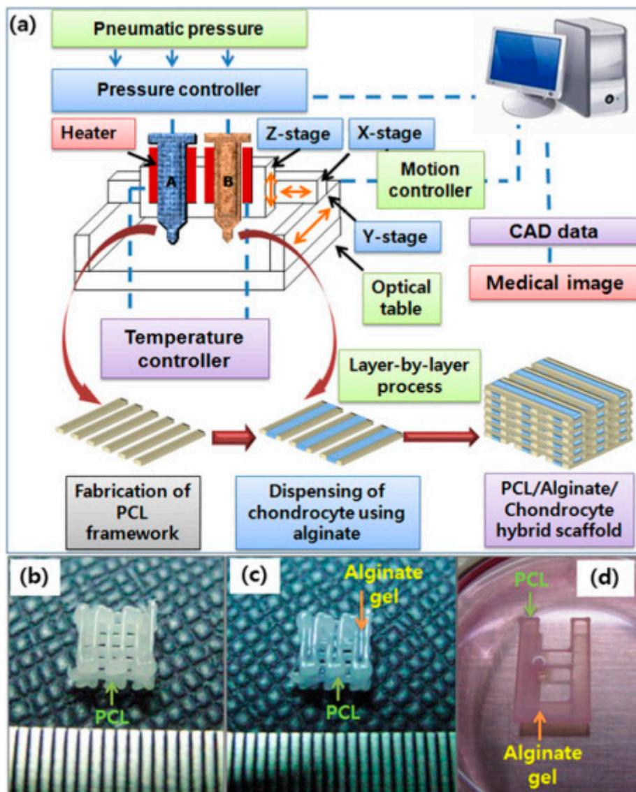
**Figure 5.** (a) Schematics of the fabrication process of cell-printed 3D polycaprolactone (PCL)–alginate gel hybrid scaffold using a multihead deposition system; Photo-images of: (b) fabricated porous 3D PCL scaffold; (c) chondrocyte-printed 3D PCL–alginate gel hybrid scaffold for in vivo experiments; and (d) simplified 2D hybrid scaffold for in vitro experiments [57].
