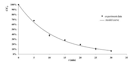
**Figure 9.** Values from the model developed in this study and from the actual experiments (reaction conditions: air pumped in at 3 mL/s,  $C_0 = 50$  mg/L,  $C_t = 600$  mg/L,  $S_L = 500$  W/m).
