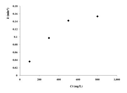
To examine the pure catalytic effect of the photocatalyst to the degradation process, the influence of the reflection and scattering of particles should be excluded. The reaction rate constant *k* in different catalyst concentrations was divided by  $I_{ave}^{0.4827}$  to exclude the influence of the reflection and scattering of catalyst.
