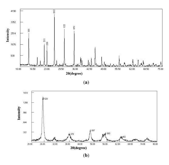
Figure 1. XRD spectra of (a) tourmaline; and (b) tourmaline-coated TiO<sub>2</sub>.
