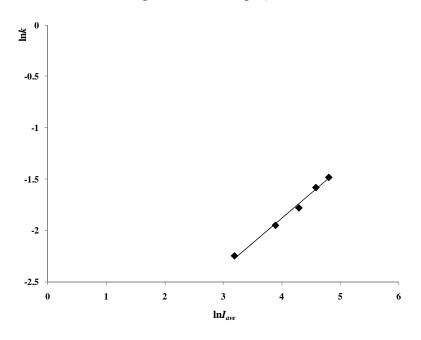
Figure 5 indicates that there is a linear relationship between  $\ln k$  and  $\ln I_{ave}$ , with a slope of 0.4827 ( $R^2 = 0.99$ ).
