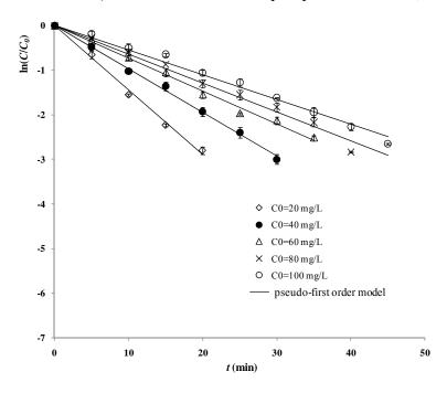
**Figure 3.** Logarithm values of 2,4-D residue ratios at different moments with various initial 2,4-D concentrations (reaction conditions: air pumped in at 3 mL/s,  $C_t = 500$  mg/L).
