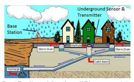
Figure 1. The architecture of urban underground IoT for wastewater monitoring.
