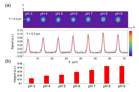
**Figure 4.** (a)  $T_1$ -weighted images of a 100-nm nanodiamond in various pH condition (top) and its signal intensity in Y = 5.3 µm plotted against X (bottom). Red line represents the fitting function, which contains seven gaussian functions. (b) Definite integrals of the fitted gaussians in each pH condition. Error bars represent the standard error of the gaussian fitting.
