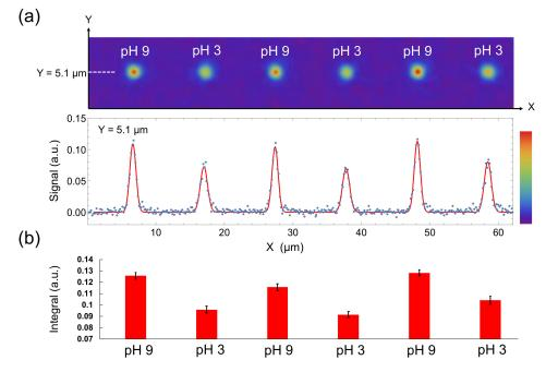
**Figure 5.** (a)  $T_1$ -weighted images of a 100-nm nanodiamond in alternately changing pH conditions (top) and its signal intensity in Y = 5.1 µm plotted against X (bottom). Red line represents the fitting function, which contains six gaussian functions. (b) Definite integrals of the fitted gaussian functions. Error bars represent the standard error of the gaussian fitting.
