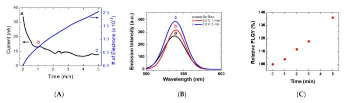
**Figure 5.** In situ photoluminescence spectra measurements under constant applied bias (+ 0.6 V) for electrodeposition of bromide on CsPbBr<sub>3</sub> perovskite film. (**A**) Current-time profiles and accumulated electron flow with time. (**B**) photoluminescence spectra of the CsPbBr3 perovskite film during the moment assigned in (**A**). (**C**) Relative PLQY enhancement with comparison of (emission peak area at time)/(emission peak area at time zero without applied bias).
