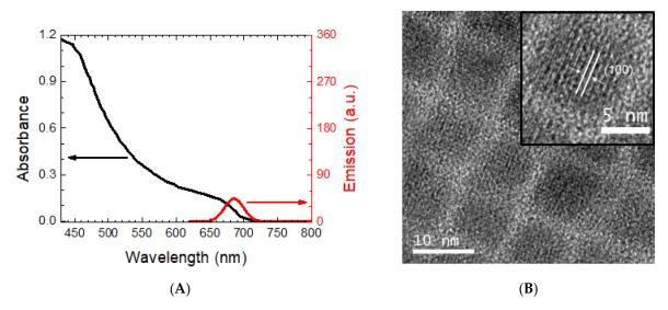
**Figure 2.** (**A**) UV-Vis. absorption (black line, left) and photoluminescence (red line, right) spectra of the CsPbI<sub>3</sub> PQDs, synthesized using Hot Water PbI<sub>2</sub>. (**B**) TEM image of the CsPbI<sub>3</sub> PQDs (inset: high resolution TEM image of single PQD with lattice fringe, which presents (100) plane of the CsPbI<sub>3</sub> structure).
