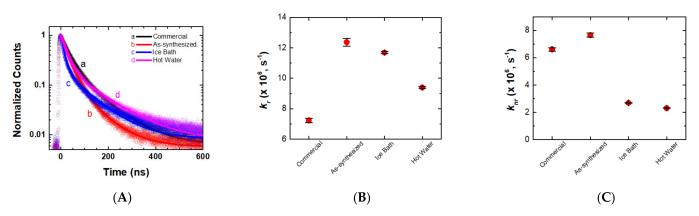
**Figure 4.** (**A**) Time-resolved photoluminescence decay kinetic traces of the four CsPbI3 PQDs made using (a) Commercial, (b) As-synthesized, (c) Ice Bath, (d) Hot Water PbI<sub>2</sub>, and their (**B**)  $k_r$  and (**C**)  $k_{nr}$ .
