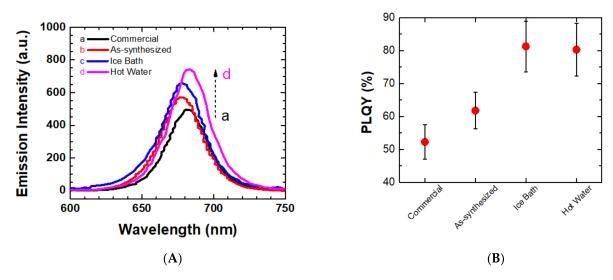
**Figure 3.** (A) Photoluminescence spectra of the four CsPbI<sub>3</sub> PQDs made using four different PbI<sub>2</sub> (a: Commercial, b: As-synthesized, c: Ice Bath, d: Hot Water PbI<sub>2</sub>). Photoluminescence spectra were taken by fixing their band edge absorption as  $0.1 \pm 0.005$ . (B) PLQY of CsPbI<sub>3</sub> PQDs made using four different PbI<sub>2</sub>.
