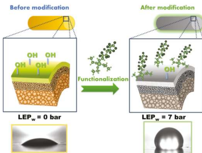
Figure 1. Ceramic membrane modification by alkylsilanes grafting agent and differences in hydrophobicity level (contact angle and water liquid entry pressure (LEP w )) before (left) and after (right) hydrophobization process.
