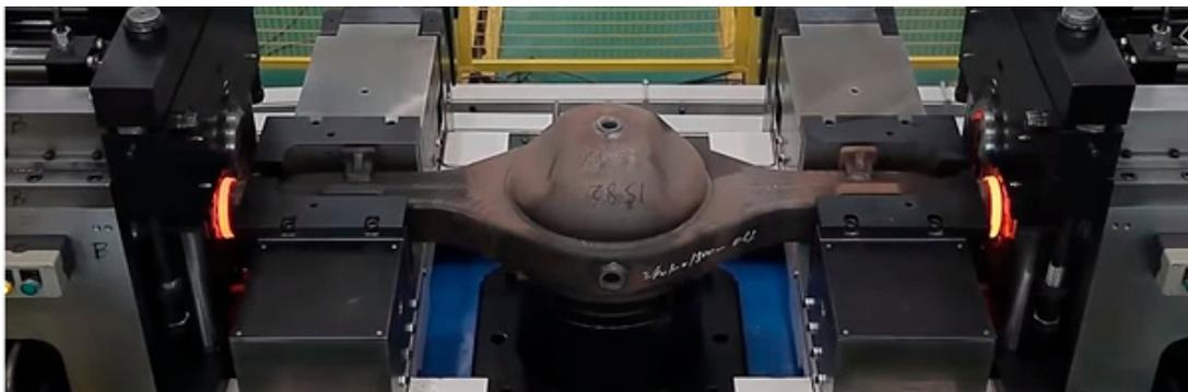
**Figure 11.** Friction welding of axles (China RCM).
