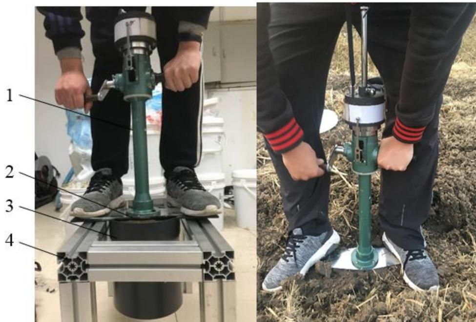
**Figure 1.** Soil penetration resistance tests in the laboratory and field. Note: 1. Soil penetrometer; 2. Remolded soil samples; 3. Container; 4. Base.
