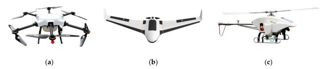
Figure 2. Multirotor (a), fixed-wing (b), and single-rotor (c) drones.
