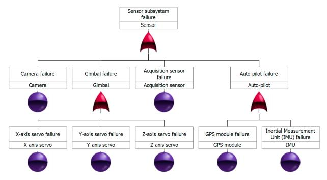
Figure 8. Fault-tree diagram of the drone's sensor subsystem.
