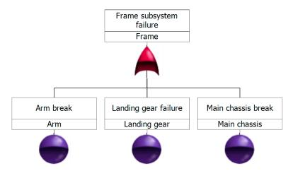
Figure 9. Fault-tree diagram of the drone's frame subsystem.
