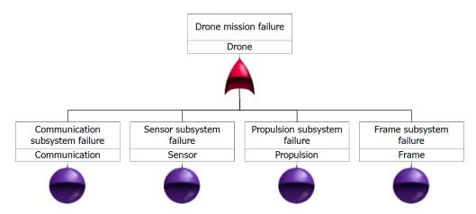
**Figure 5.** A fault-tree diagram of a drone prototype system.
