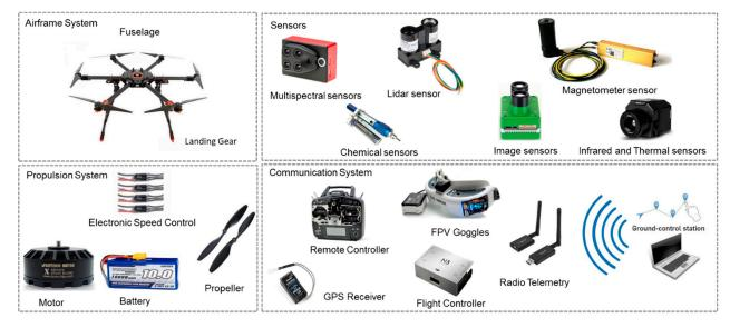
Figure 4. Subsystems and components of our drone prototype for inspecting wind turbines.
