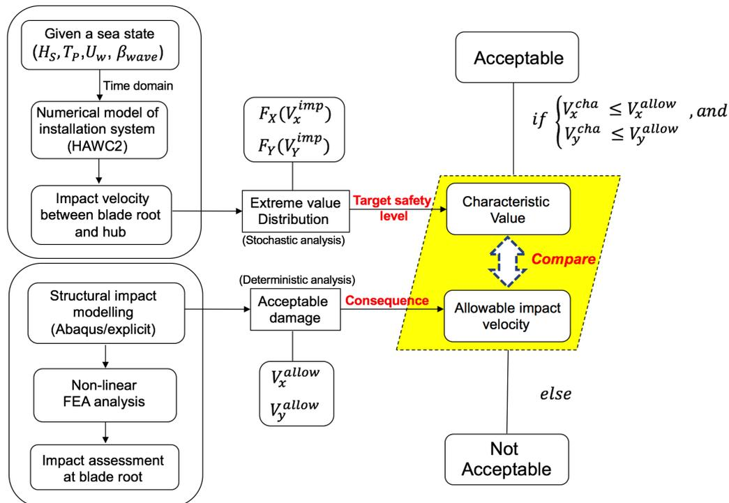
Figure 5. Response-based methodology for estimating operational limits for blade-root mating task.
