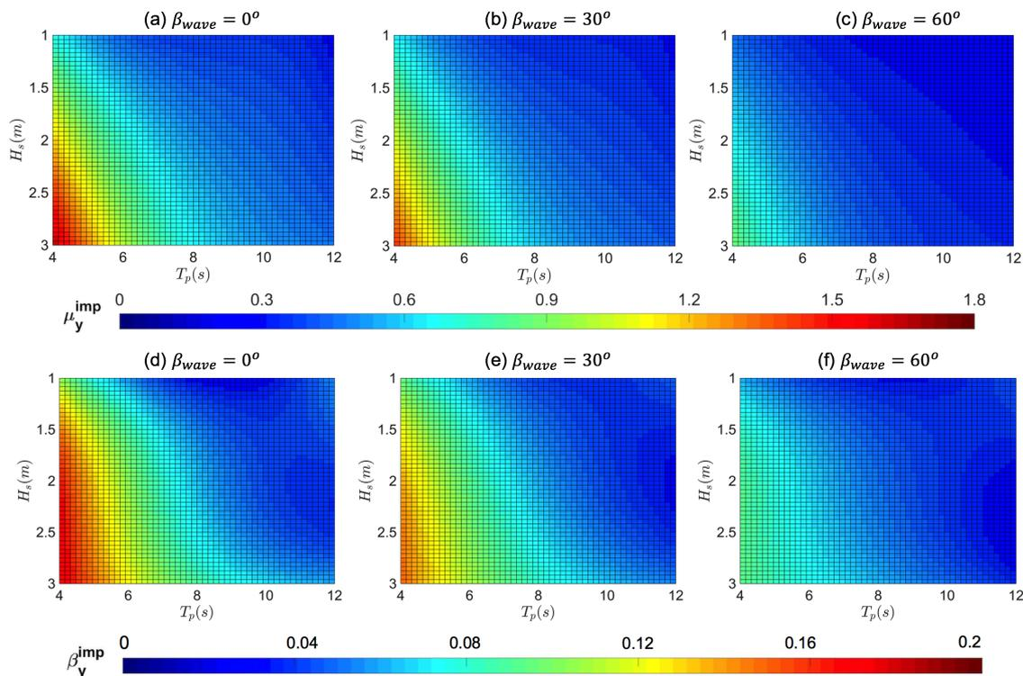
**Figure 13.** 2D-response surface contour plot for Gumbel parameters ( $\mu_y^{imp}, \beta_y^{imp}$ ) for load case  $H_s = 2$  m,  $T_p = 4$  s,  $U_w = 6$  m/s:  $\mu_y^{imp}$ : (a)  $\beta_{wave} = 0^\circ$  (b)  $\beta_{wave} = 30^\circ$  (c)  $\beta_{wave} = 60^\circ$ ;  $\beta_y^{imp}$ : (d)  $\beta_{wave} = 0^\circ$ ; (e)  $\beta_{wave} = 30^\circ$ ; (f)  $\beta_{wave} = 60^\circ$
