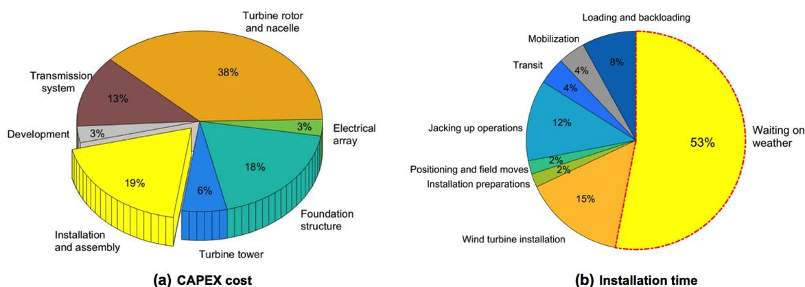
**Figure 1.** (a) Cost breakdown for different components of *CapEx* for OWT project; (b) contribution of different activities during installation and assembly activities (statistics based on 2016–2017 data from [5,7]).
