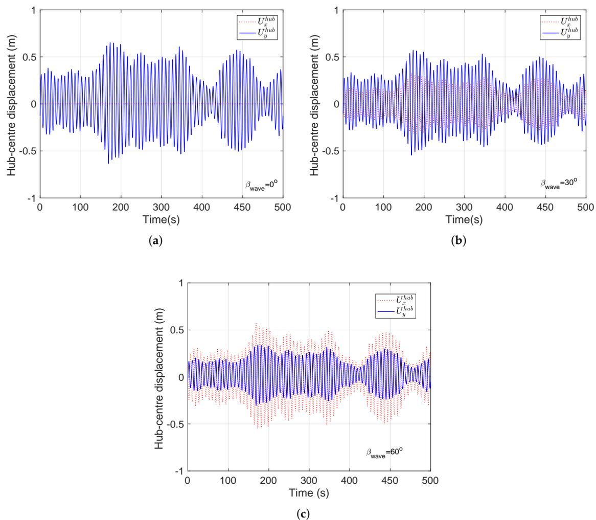
**Figure 8.** Displacement of the hub-center in side-side ( $U_x^{hub}$ ) and fore-aft directions ( $U_y^{hub}$ ) for  $H_s = 2$  m,  $U_w = 8$  m/s,  $T_p = 4$  s (a)  $\beta_{wave} = 0^\circ$  (b)  $\beta_{wave} = 30^\circ$  (c)  $\beta_{wave} = 60^\circ$ .
