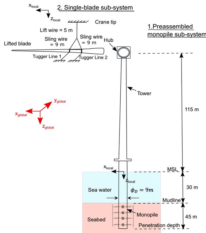
Figure 6. Numerical modelling of installation system in HAWC2.
