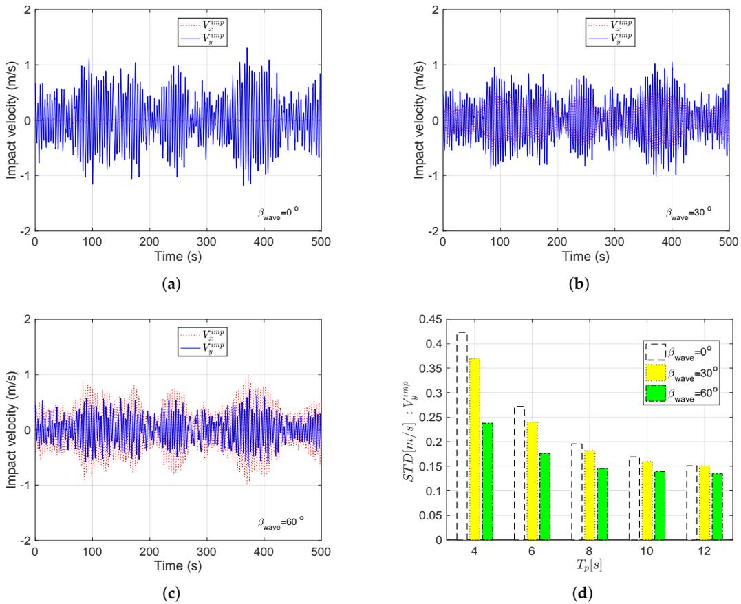
**Figure 10.** Response-time histories for  $V_x^{imp}$  and  $V_y^{imp}$  for load case  $H_s = 2$  m,  $T_p = 4$  s,  $U_w = 8$  m/s and for different wind-wave misalignment (a)  $\beta_{wave} = 0^\circ$  (b)  $\beta_{wave} = 30^\circ$  (c)  $\beta_{wave} = 60^\circ$  (d) comparison of standard deviations for  $V_y^{imp}$  for different  $T_p = 4$  s, 6 s, 8 s, 10 s, and 12 s.
