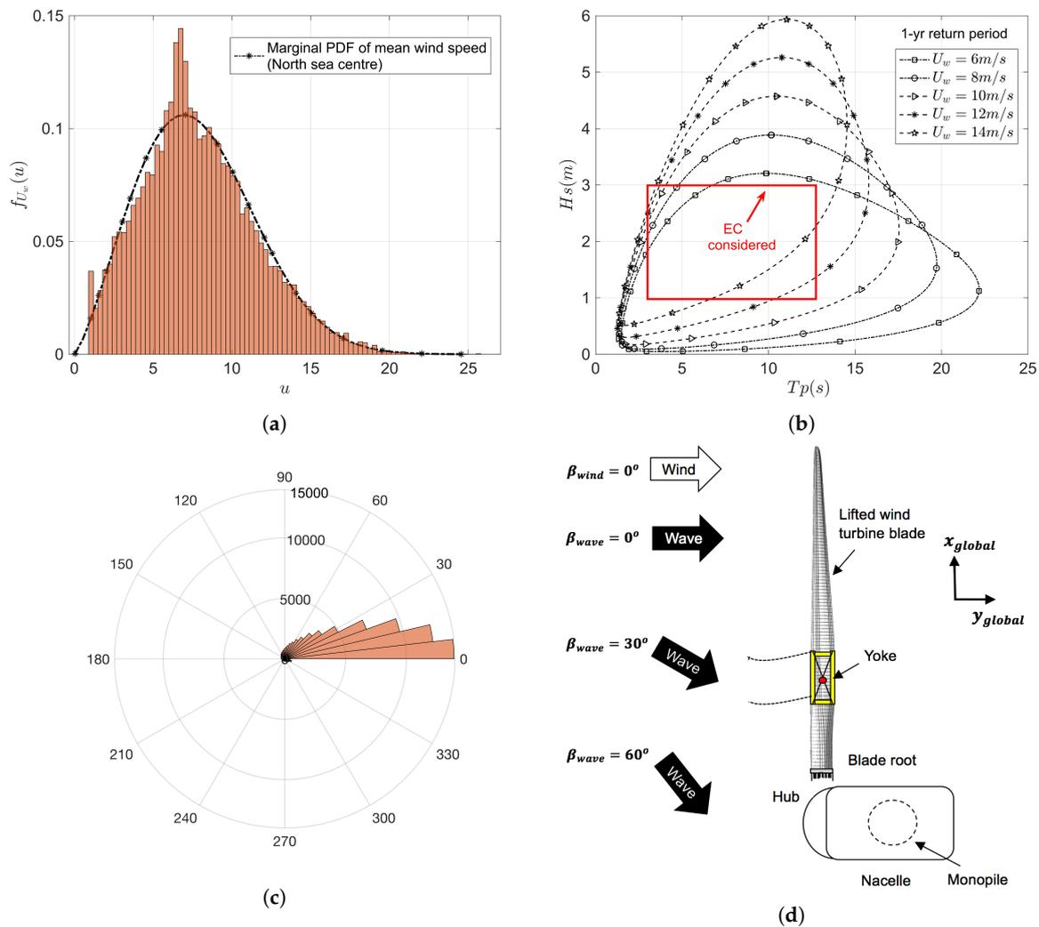
**Figure 7.** Description of North sea center offshore site (a) marginal PDF of mean wind speed ( $f_{U_w}(u)$ ) (b) 2D-contour surface for  $H_s$ - $T_p$  for different ranges of wind speeds (c) wind–wave misalignment ( $\beta_{wave}$ ) (d) bird view of wind-turbine blade-root mating task.
