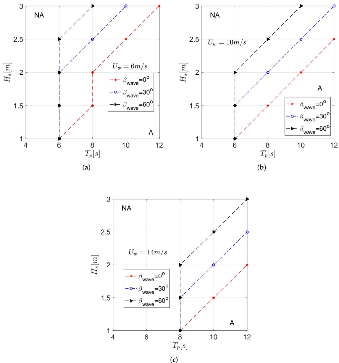
**Figure 16.** Operational limiting sea state curves for different  $H_s$ ,  $T_p$ ,  $U_w$ ,  $\beta_{\text{wave}} = 0^\circ, 30^\circ, 60^\circ$  with specific: (a)  $U_w = 6 \text{ m/s}$  (b)  $U_w = 10 \text{ m/s}$  (c)  $U_w = 14 \text{ m/s}$  (A: Acceptable domain and NA: Not acceptable domain for the mating task).
