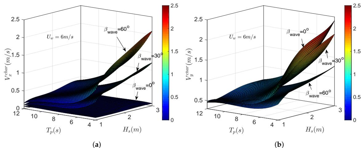
**Figure 15.** Response surface for (a)  $V_x^{char}$  and (b)  $V_y^{char}$  for different  $H_s, T_p, \beta_{wave} = 0^\circ, 30^\circ, 60^\circ$  and  $U_w = 6$  m/s.
