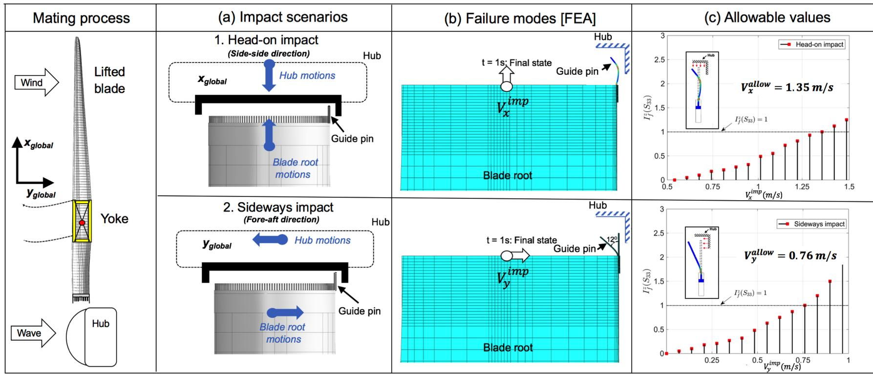
Figure 4. Critical event of blade-root impact with hub during mating: (a) impact scenarios, (b) failure modes at the blade root and (c) allowable impact velocities [42].
