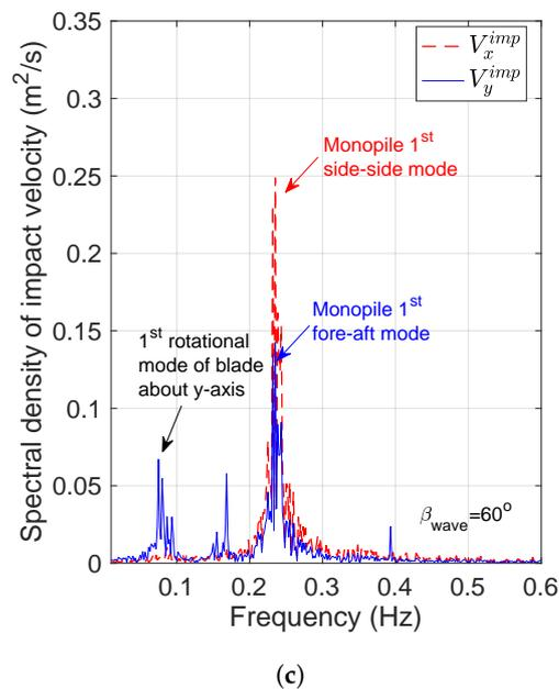
**Figure 11.** Spectral density curve for  $V_x^{imp}$  and  $V_y^{imp}$  for load case  $H_s = 2$  m,  $T_p = 4$  s,  $U_w = 8$  m/s and for different wind–wave misalignment (a)  $\beta_{wave} = 0^\circ$  (b)  $\beta_{wave} = 30^\circ$  (c)  $\beta_{wave} = 60^\circ$ .
