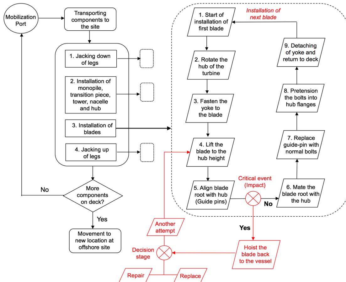
Figure 3. Detailed procedure involved during blade-root mating task.
