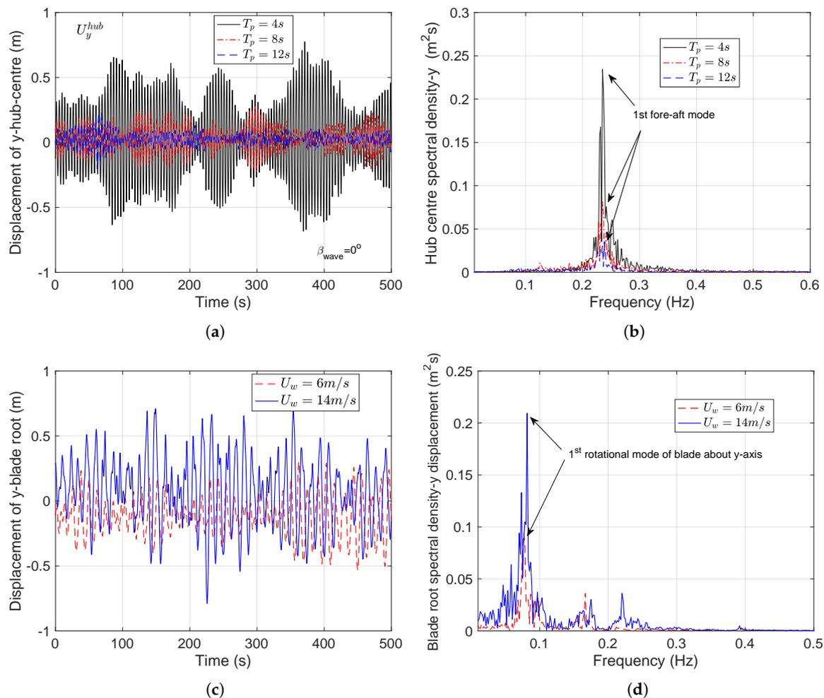
**Figure 9.** (a) Displacement hub-center y displacement ( $U_y^{hub}$ ) (b) Spectral densities (c) Blade root y displacement (d) Spectral densities.
