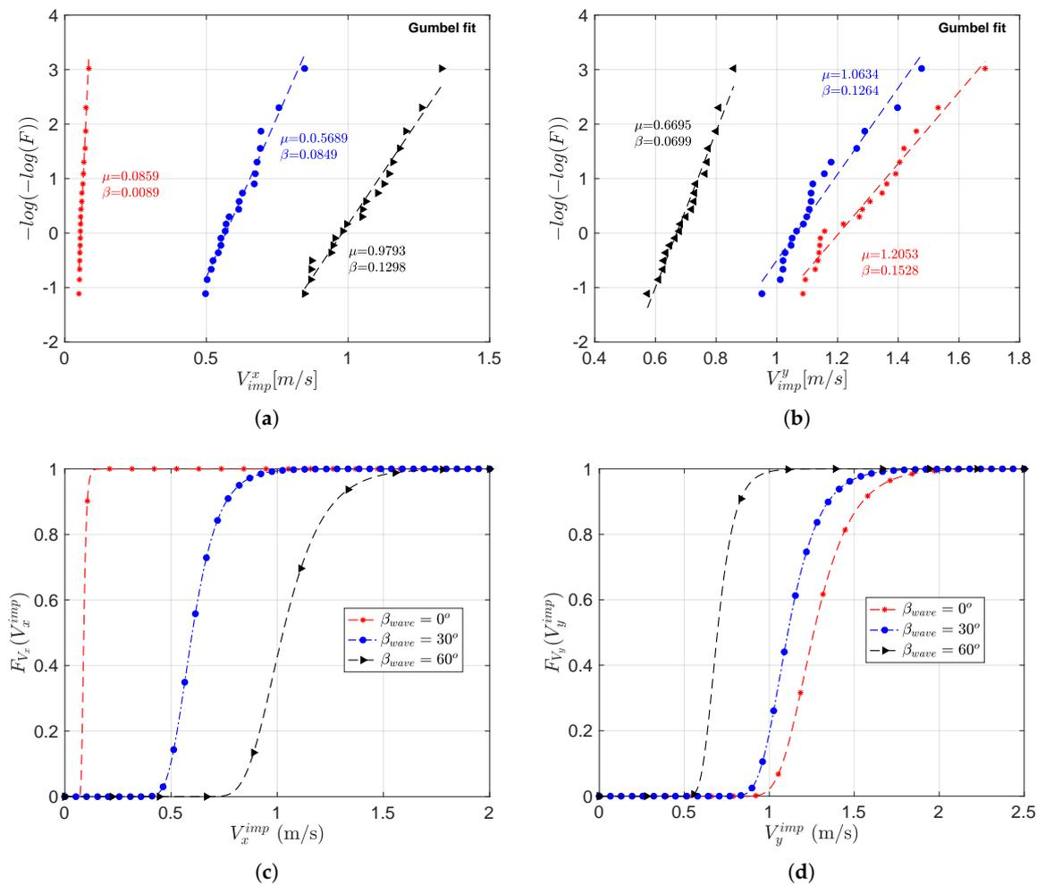
**Figure 12.** Fitting of the extreme (a)  $V_x^{imp}$  (b)  $V_y^{imp}$  to the Gumbel probability paper; (c)  $F_{V_x}(V_x^{imp})$  (d)  $F_{V_y}(V_y^{imp})$  for  $H_s = 2$  m,  $T_p = 4$  s,  $U_w = 8$  m/s and for different wind–wave misalignment  $\beta_{wave} = 0^\circ, 30^\circ$  and  $60^\circ$ .
