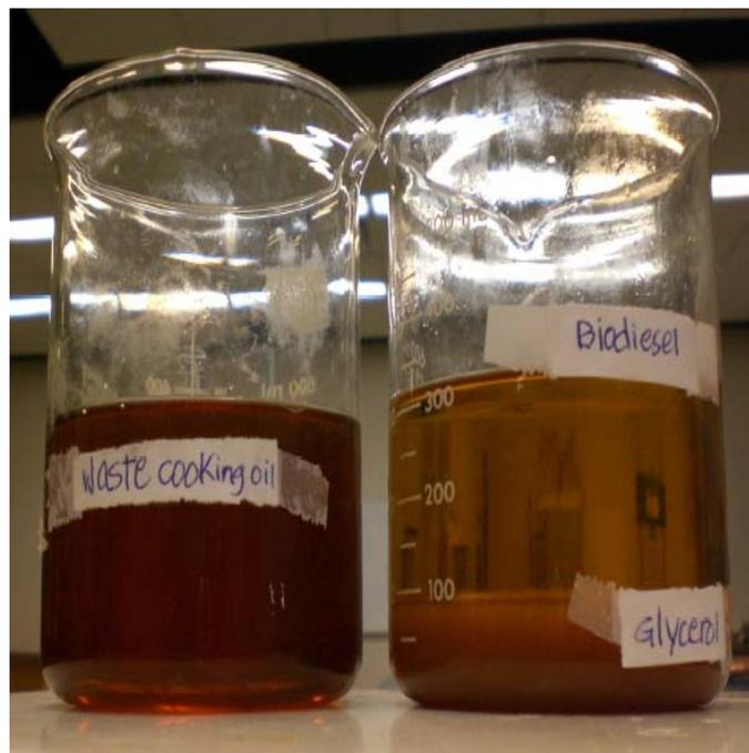
Figure 7 shows the glycerin biodiesel separation by gravity method. The biodiesel was separated in another vessel for washing. It was washed using a separating funnel creating a fine mist of water from the top (Figure 8).
