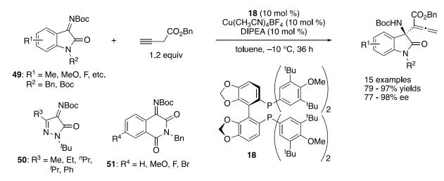
**Scheme 42.** Cu(I)-catalyzed asymmetric  $\alpha$ -allenylation of activated ketimines.
