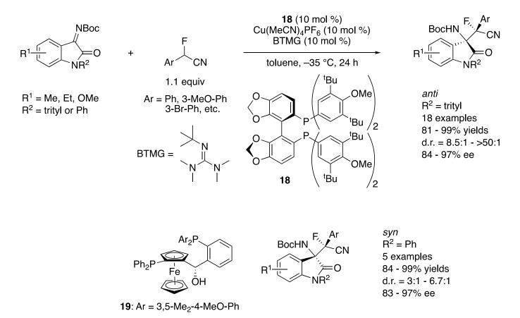
**Scheme 18.** Stereodivergent asymmetric Mannich reaction of  $\alpha$ -fluoronitriles with isatin-derived ketimines.
