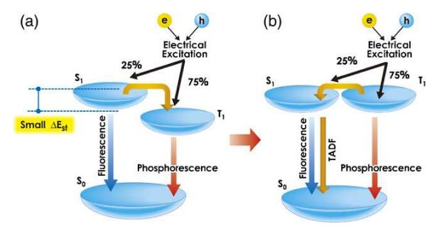
**Figure 1.** Light generation processes in **(a)** fluorescence and phosphorescence-based organic light-emitting diodes (OLEDs) and **(b)** thermally activated delayed fluorescence (TADF)-based OLEDs. Figure reproduced with permission from Adachi et al. [54] (reproduced with permission from [54]. Copyright The Japan Society of Applied Physics, 2014).
