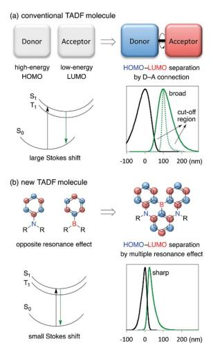
**Figure 7.** Comparative representation of energy diagram for a traditional TADF emitter (**a**) and the design developed to generate a multiple resonance effect (**b**). The curve corresponding to the emission spectrum of a benchmark blue OLED is provided as the green dotted line. Figure reproduced with permission from Hatakeyama et al. [95] (reproduced with permission from [95] Copyright Wiley-VCH, 2016).
