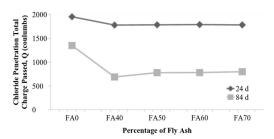
Fig. 8. Chloride penetration with time
