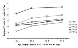
Fig. 2. Indirect tensile strength gain with time
