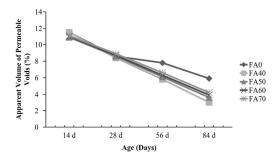
Fig. 5. Apparent volume of permeable voids with time
