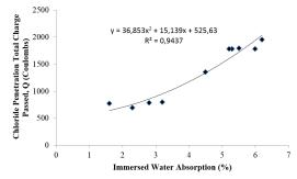
Fig. 10. Immersed Water Absorption vs. Chloride Penetration
