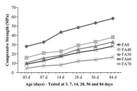
**Fig. 1.** Compressive strength gain with time
