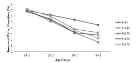
Fig. 4. Immersed water absorption gain with time
