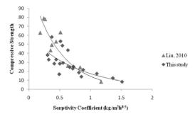
Fig. 7. Compressive strength with sorptivity
