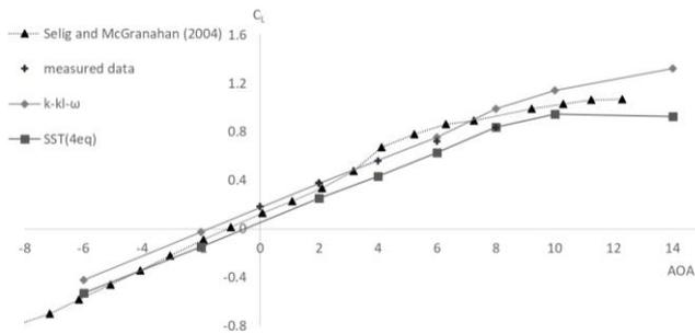
Figure 4: Lift coefficient versus angle of attack for Re number of 200,000 for the NRL S834 airfoil
