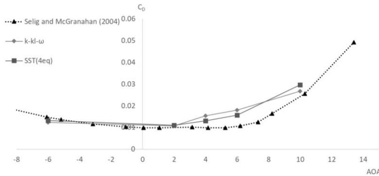
Figure 7: Drag coefficient versus angle of attack for Reynolds numbers 350,000 for the NRL S834 airfoil
