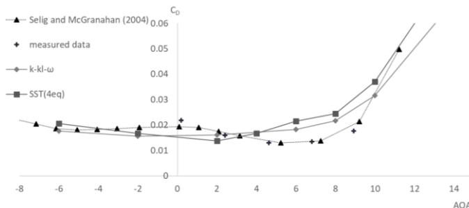
Figure 5: Drag coefficient versus angle of attack for Reynolds numbers 200,000 for the NRL S834 airfoil
