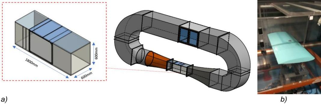
Figure 1: (a) The wind tunnel facility of the AUTH and (b) The constructed NRL S8334 airfoil, mounted inside the windtunnel
