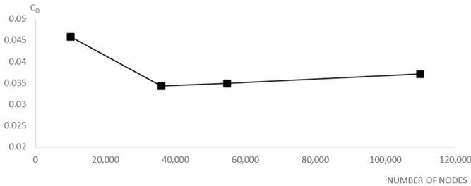
Figure 3: Grid dependency study (Coefficient of Drag)
