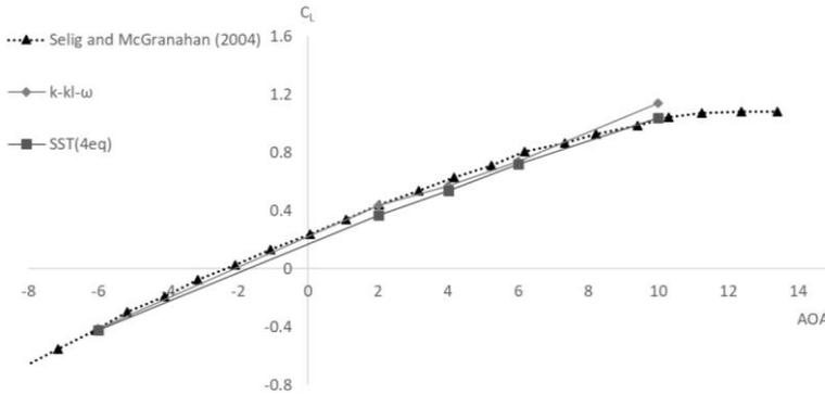
Figure 6: Lift coefficient versus angle of attack for Reynolds numbers 350,000 for the NRL S834 airfoil
