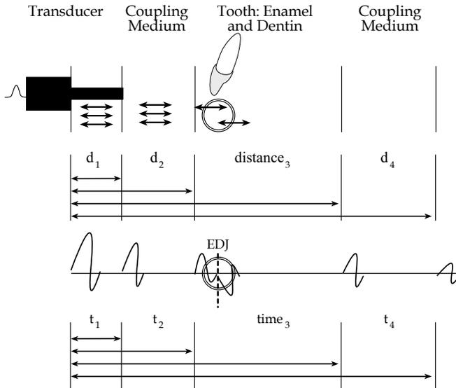
**Fig. 1.** Schematic illustration of the ultrasound pulse-echo technique. The circled regions indicate phase inversion. Orientation of the tooth relative to the transducer sensor beam is important because ultrasound waves will especially deviate when meeting a curved surface. Accordingly, specimens were placed in the test chamber with the most flat crown surface facing the sensor tip. Because only single-rooted teeth were studied, this common was the labial or buccal surface of the tooth.
