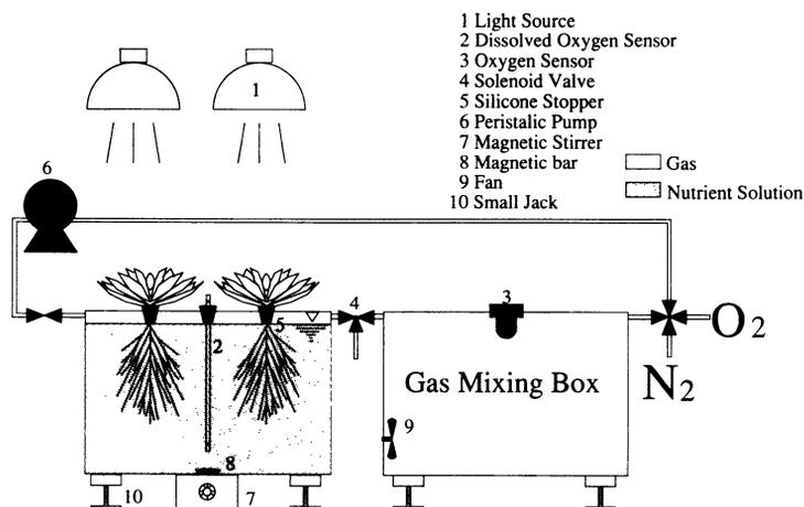
**Fig. 1** A schematic diagram of an airtight hydroponic system for the measurement of root respiration under various DO concentrations.
