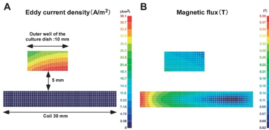
**Fig. 4.** Calculated distributions of the magnetic flux and the eddy current during magnetic stimulation (0.25T) of the system described in Fig. 4.<sup>32</sup> (A) Eddy current density, (B) magnetic flux. The calculated magnetic flux was 0.11 to 0.18T and eddy current, 26.8 to 38.1 A/m<sup>2</sup>, within the culture medium. © 2006IEEE
