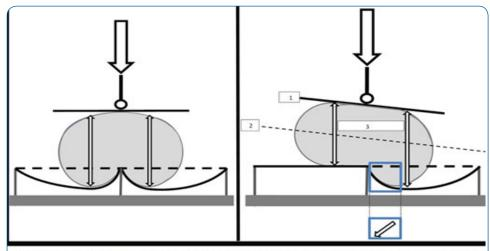
Figure 1: Comparison of the squashing of a ball by an articulated piston against two elastic structures.
