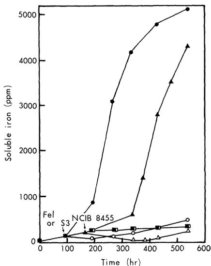
Fig. 4. Effect of *T. ferrooxidans* and *T. thiooxidans* on oxidation of Yanahara pyrite: Release of soluble iron from pyrite.
