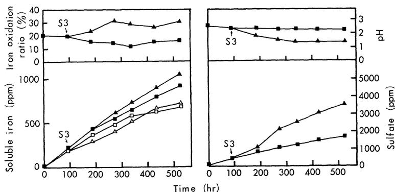
Fig. 3. Effect of *T. thiooxidans* on oxidation of Matsuo pyrite: Release of soluble iron and sulfate from pyrite and changes in iron oxidation ratios and pH values.
