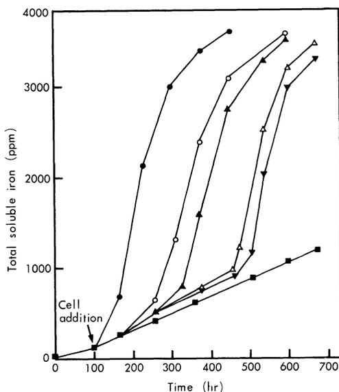
Fig. 7. Effect of mixed addition of *T. ferrooxidans* and *T. thiooxidans* on pyrite oxidation.
