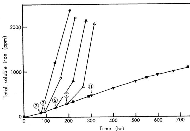
Fig. 5. Effect of varying the cell age of *T. ferrooxidans* on pyrite oxidation.
