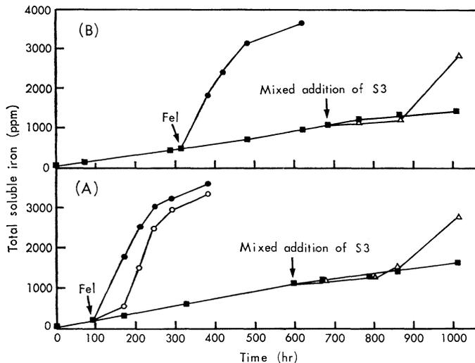
Fig. 6. Effect of varying the inoculum size of 2-day (A) and 11-day (B) cultured *T. ferrooxidans* and mixed addition of *T. thiooxidans* on pyrite oxidation.
