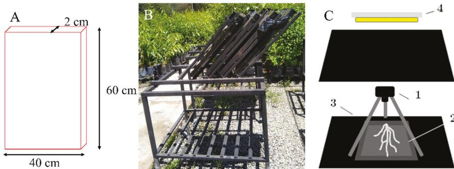
**Figure 6.** Rhizobox structure and dimensions used to evaluate root system architecture traits (A); angle and position of rhizobox in the field experiment (B); rhizobox (2) placed horizontally on a black surface (3) at a distance of ~134 cm from the digital camera (1) to avoid the effect of light (4) (C).
