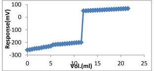
Chart (6): Titration curve for sample ( $1 \times 10^{-3}M$ ) PCH with ( $1 \times 10^{-3}M$ ) MP standard by electrode E1.
