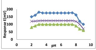
Chart (3): Response of pH effect for (PCH) electrodes at concentration  $10^{-3}$  M of pilocarpine hydrochloride solution,  $\blacksquare$  $E_{1,\times} E_{2,} \blacktriangle E_{5}$ .
