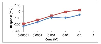
Chart (4): Interfering  $K^{+1}$  by separation method for (PCH+MP+DBPH) membrane,  $\blacksquare$  -pilocarpine hydrochloride solution,  $\blacksquare$  -solution of  $K^{+1}$ .
