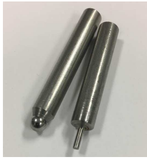
Figure 3.3: Spherical and flat-end indenters.
