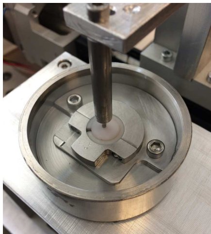
Figure 4.1: Indentation test performed on osteochondral bovine disk.
