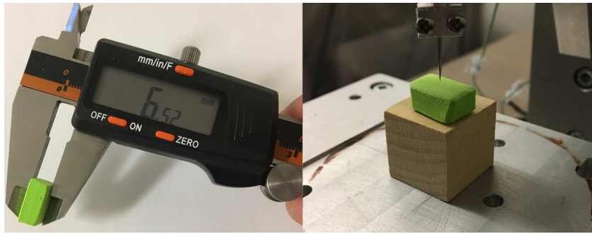
Figure 3.15: Measurement of rubber block thickness by digital caliper (Left) and by needle penetration test (Right).
