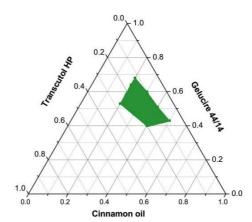
Fig. 4: Ternary phase diagram of SEDDS between cinnamon oil, gelucire 44/14 and transcutol HP (green domain indicates the region of self emulsification
