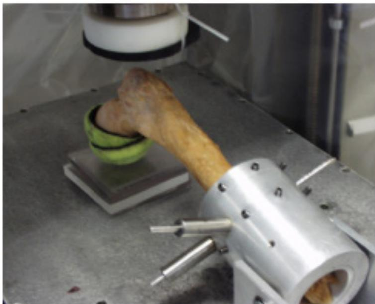
**Fig. (1).** Mechanical testing setup of the proximal femur that simulates a sideways fall on the greater trochanter. The femoral shaft was positioned at 10° from horizontal axis, and neck at 15° internal rotation. Two halves of tennis ball were used to simulate cartilage contact in the femoral head. The load was applied to the greater trochanter through a pad simulating soft tissue, using a constant loading speed of 6.6 mm/second.
