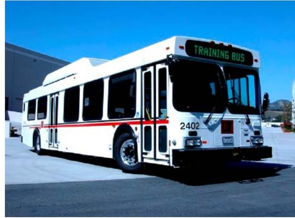
**Fig. 21. Gasoline/electric hybrid bus with an electrochemical capacitor energy storage system.**
