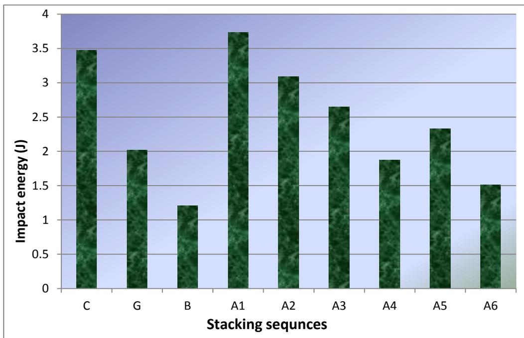
**Fig. 14.** Effect of stacking sequences of hybrid laminate composites on the impact energy
