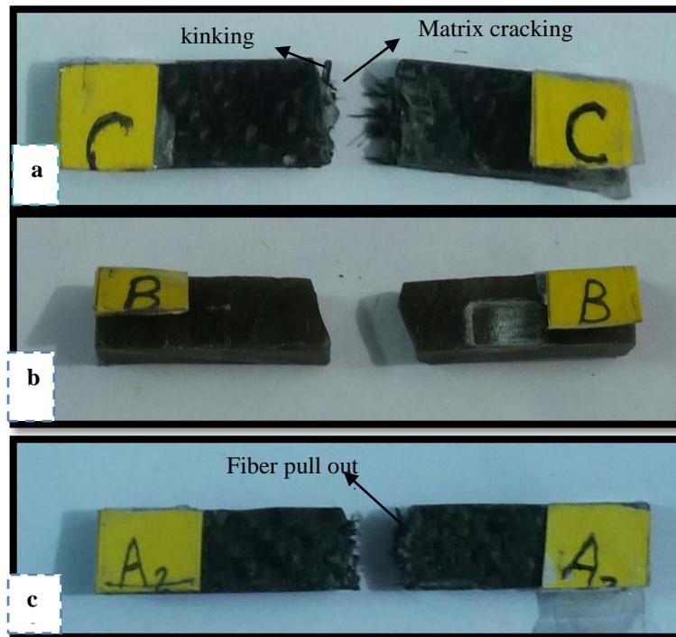
**Fig. 13.** Photographs of a) CFRP, b) BFRP and stacking sequence codes and c) A2 hybrid laminate composites specimens after the Charpy impact test
