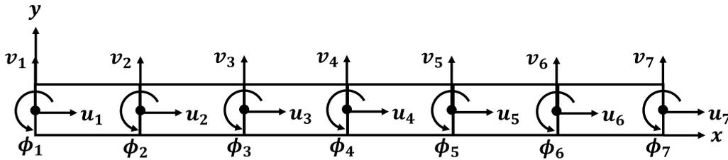
Fig. 7. Finite element model for hybrid composite beam.
