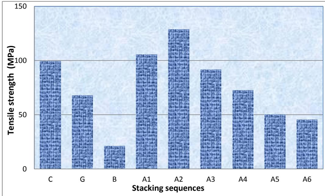
**Fig. 9. Effect of stacking sequences of hybrid laminate composites on the tensile strength.**
