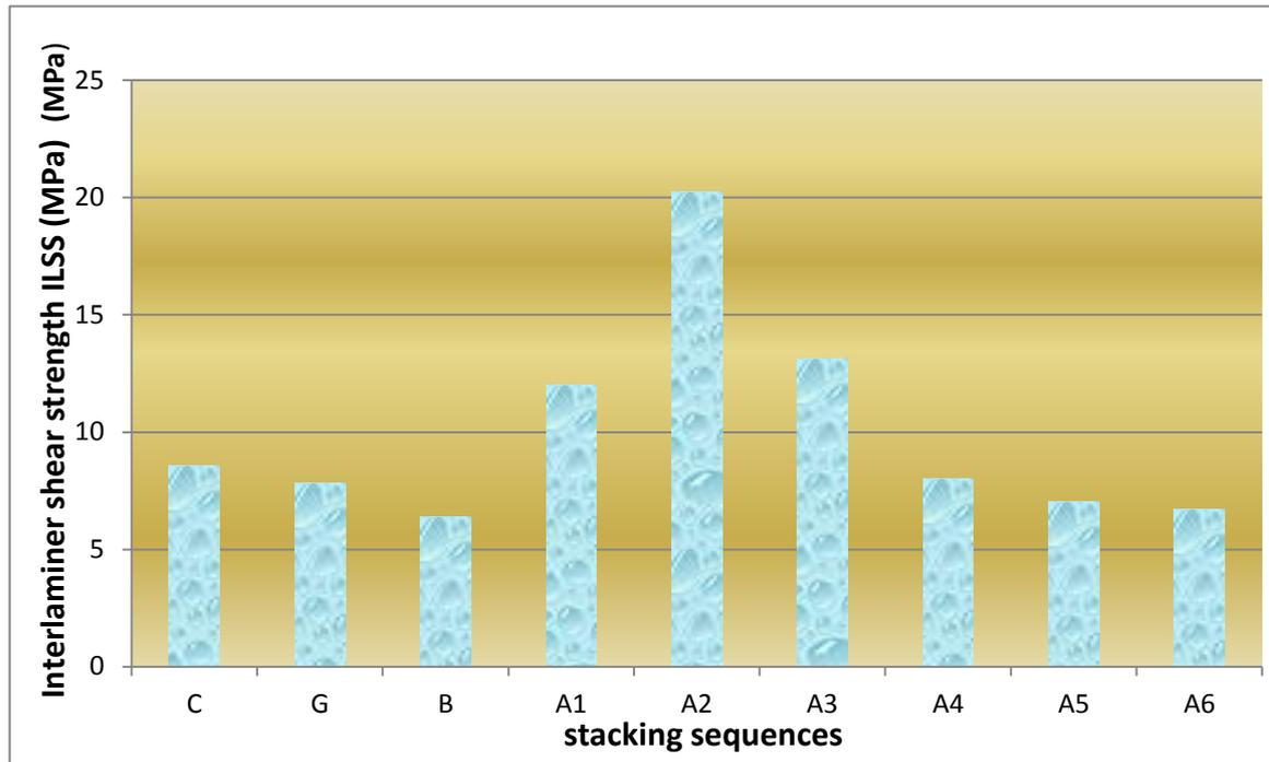
**Fig. 12. Effect of stacking sequences of hybrid laminate composites on the interlamier shear strength (ILSS)**
