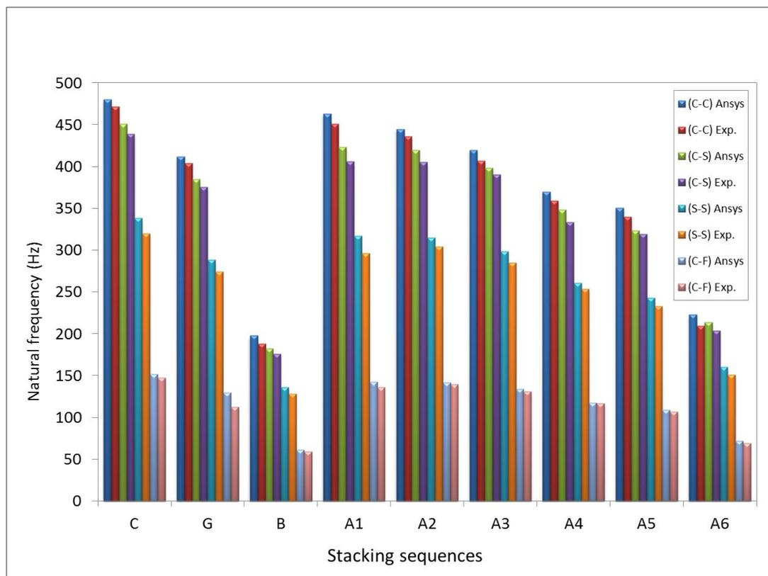
**Fig. 15. Natural frequency at different boundary fixations and various stacking sequences**
