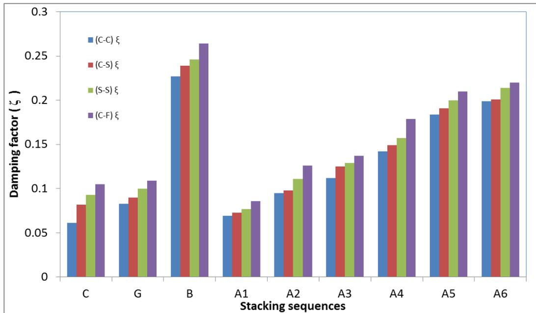
**Fig. 16. Damping factor at different boundary fixations and various stacking sequences**
