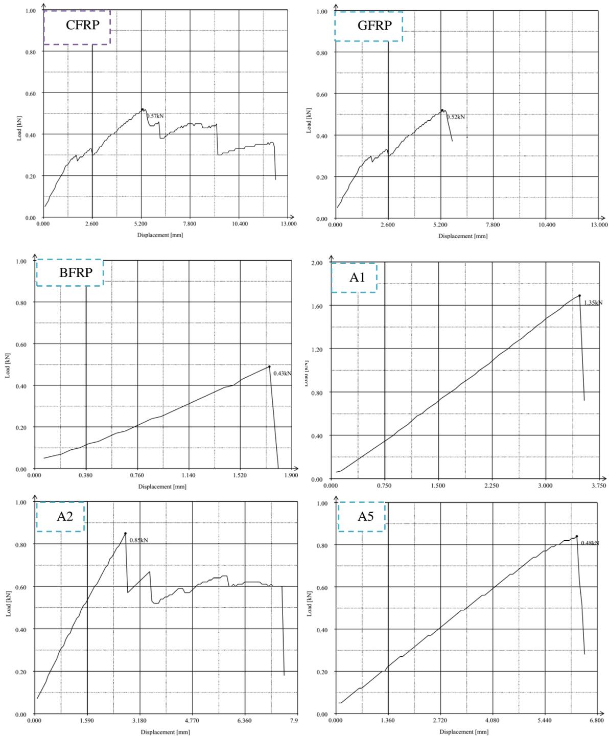
**Fig. 10. Load displacement graphs of bending test for CFRP, GFRP, BFRP and some codes A1, A2, A5 hybrid laminate composites.**
