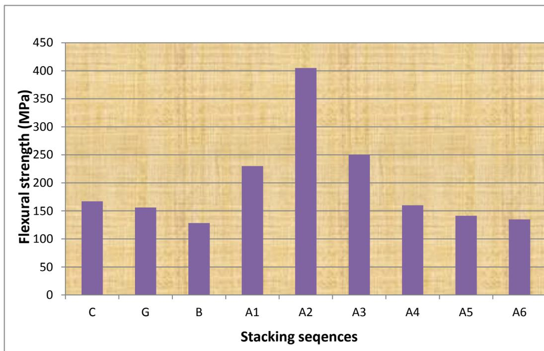
**Fig. 11. Effect of stacking sequences of hybrid laminate composites on the flexural strength**
