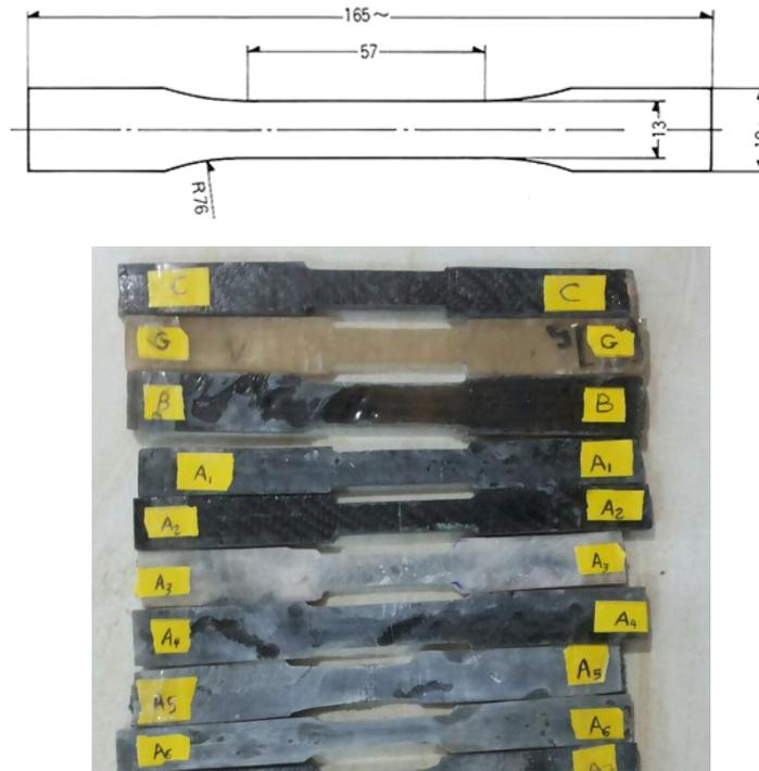
**Fig.3. Tension test specimens of composites and hybrid laminate composites**
