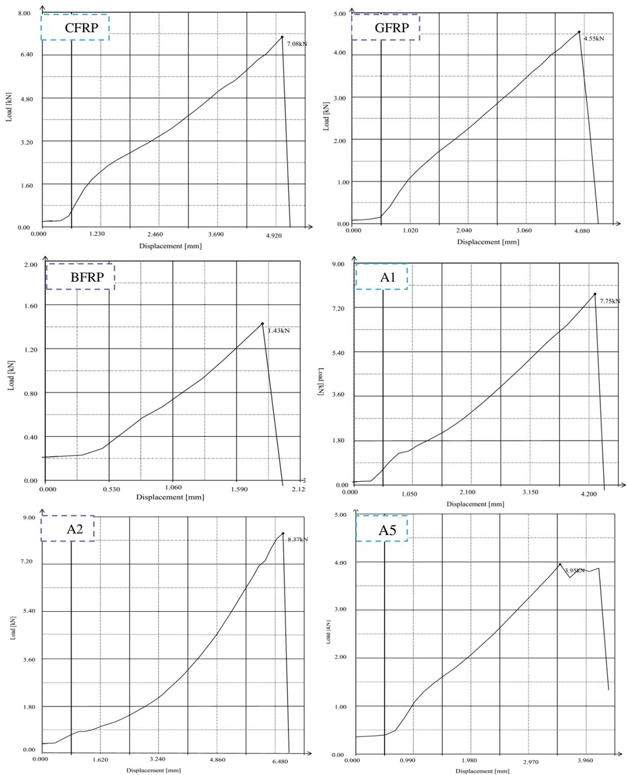
**Fig. 8. Load displacement graphs of tension test for CFRP, GFRP, BFRP and some codes A1, A2, A5 hybrid laminate composites.**
