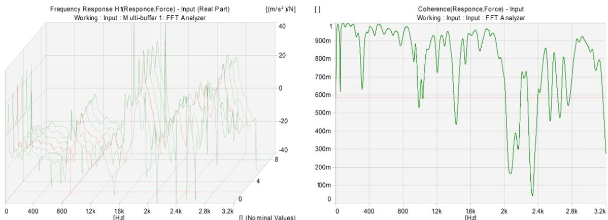
**Fig.5. A sample of frequency response function and coherence function for hybrid laminates composite specimen with code A1 at clamped-simple supported.**
