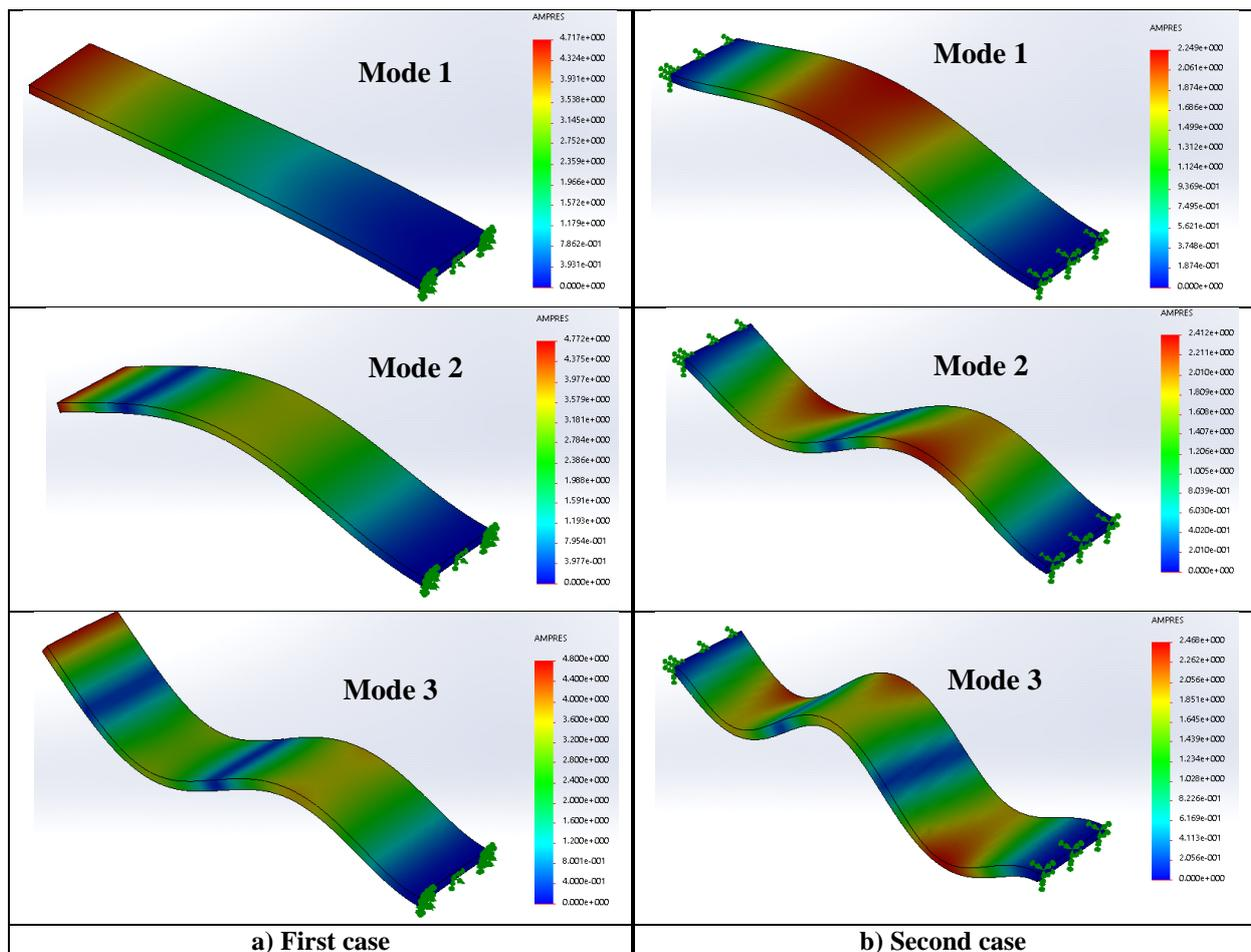
**Fig. 17. Mode shapes of the hybrid laminate composites code A2 for a) First case (Clamped-Free) and b) Second case (Clamped-Clamped)**
