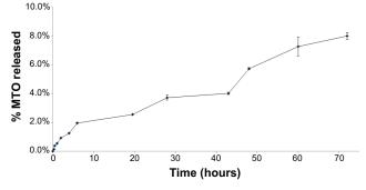
**Figure 11** Release kinetics of MTO from SEON<sup>LA-BSAKMTO</sup> in PBS at 37°C. **Notes:** No burst release was observed; MTO is slowly released with linear kinetics. After 72 hours, only 8.01%±0.24% of the original amount of MTO is located outside the membrane. In the lysate of particle suspension after 72 hours, we detected 93.38%±2.72% of the original amount of MTO. All measurements were performed in triplicate.
