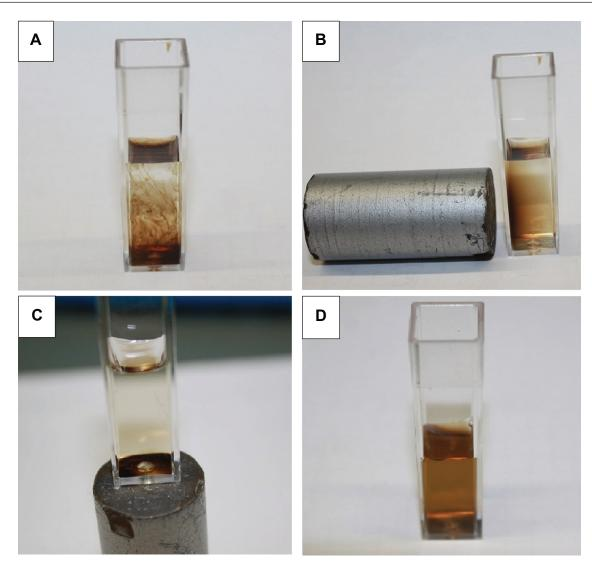
Figure 6 Manipulation of 20  $\mu L$  of SEON^{LA-BSA} particles in 2 mL of water with a magnet.
