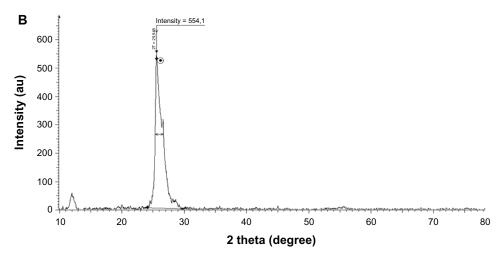
Figure 3 X-ray diffraction patterns of (A) graphene oxide and (B) bacterially reduced graphene oxide.
