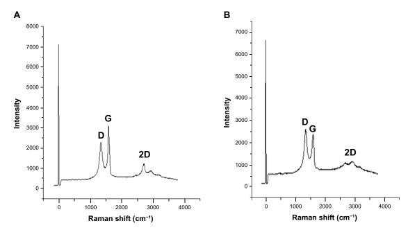
Figure 6 Raman spectra of (A) graphene oxide and (B) bacterially reduced graphene oxide.
