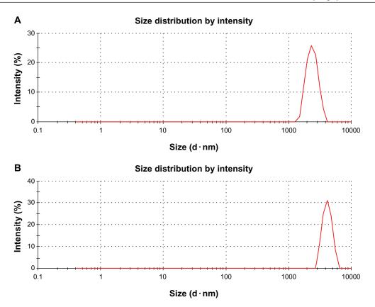
Figure 4 Hydrodynamic size distribution of (A) graphene oxide and (B) bacterially reduced graphene oxide (500 μg/mL) measured by dynamic light scattering at room temperature in deionized water.
