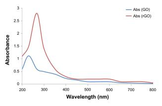
**Figure 2** Ultraviolet–visible absorption spectra of graphene oxide (GO) and the reduced graphene oxide (rGO) suspension reduced by bacterial biomass (50  $\mu$ g/mL). **Abbreviation:** Abs, absorption spectrum.
