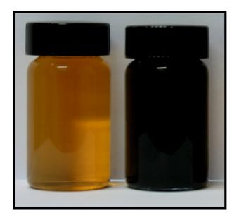
Figure 1 Photograph of graphene oxide (left) and bacterially reduced graphene oxide (right) at a concentration of 500  $\mu$ g/mL.
