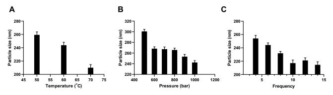
Figure 2 Investigation of the homogenization process with different (A) temperatures, (B) pressures, and (C) frequencies.
