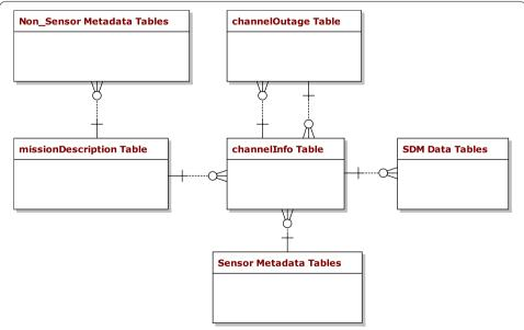
**Fig. 1** Relational PNT Database Overview: Every row in missionDescription Table is an independent data log in the SDM format which is uploaded in the database. The SDM tables contain all of the navigation data associated with the data logs
