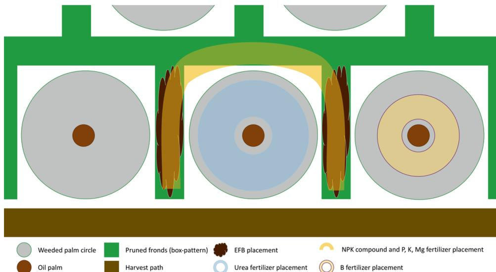
**Photo 17.** In mature oil palms, fertilizers should be applied to ‘target areas’, where nutrient uptake is most effective and losses are minimized.
