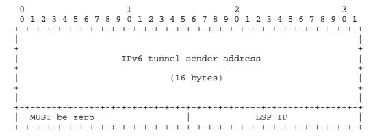
IPv6 tunnel sender address
