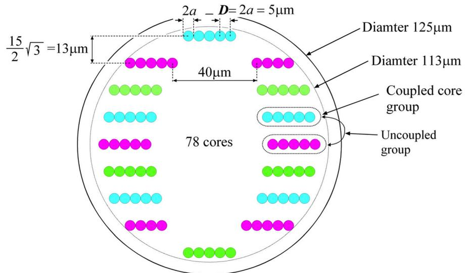
(b) hybrid configuration of coupled homogeneous multi-core and uncoupled heterogeneous multi-core fibers
