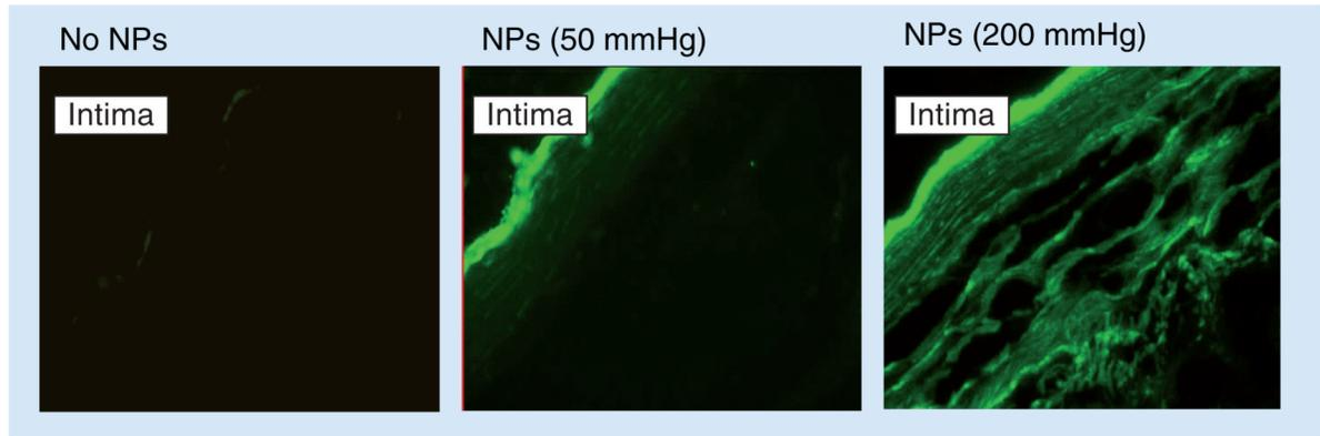
**Figure 2. Delivery of poly(lactic-co-glycolic acid) nanoparticles to a tissue engineered vascular graft (decellularized and heparin covalently linked porcine carotid artery graft)**
